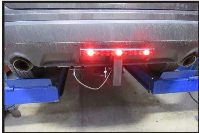
5. Connect the 4-flat on the light bar to the 4-flat on the wiring harness. Check the operation of all signals.
