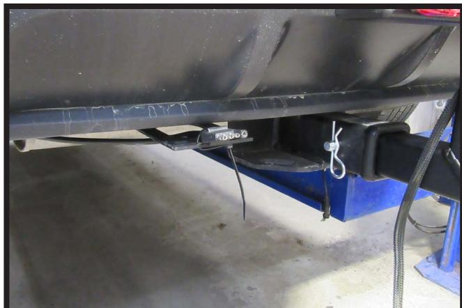
3. Attach 4-flat plug to receiver hitch with cable tie(s) and route the wiring harness to the front of the vehicle. Secure any excess wiring out of the way using provided cable ties.
