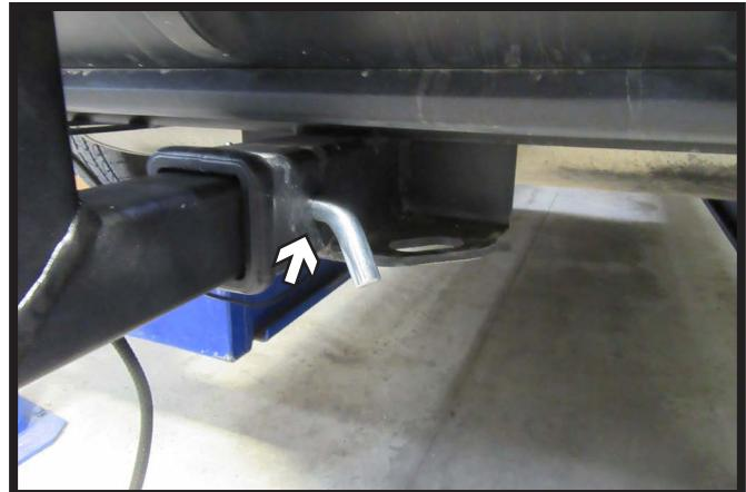
2. Secure light bar to hitch using the provided pin and clip.
