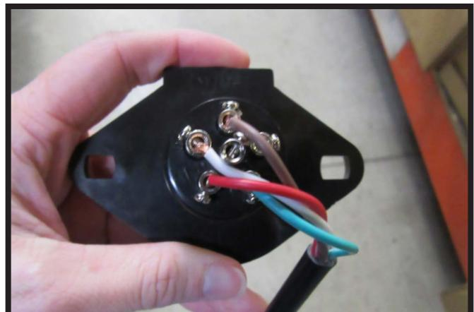
4. Install the harness wires to the plug on the front of the vehicle. Reference wiring diagram on page 2.
