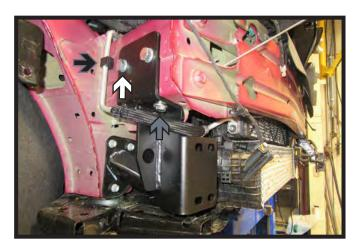
18. Install a 1/2" bolt with lock washer and whiz nut into the back side hole (white). Then install a 3/8" bolt with lock washer and nut plate in front bottom hole (gray). Tighten. Re-clip rear line to the frame (black).
