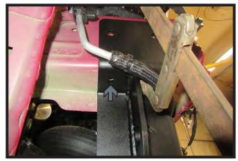
15. Raise the passenger side plate into place on the vehicle ensuring that it is as high as possible and the front side is against the flange on the frame. Hold in place with vise grips. Using a 1/2" drill bit, drill the front side hole (white) using the baseplate as a template. Then using a 3/8" drill bit, drill the back bottom hole using the baseplate as a template (gray).
