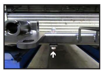
22. Loosely install support bracket to the bottom of the cross member using a 1/2" x 3-1/2" bolt with lock washer, spacer tube, flat washer and lock nut. Do this on both sides of the vehicle
