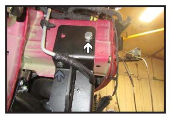
16. Install a 1/2" bolt (white) with lock washer and whiz nut into the front side hole. Then install a 3/8" bolt (gray) with lock washer and whiz nut in back bottom hole. Tighten.
