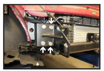
19. Hold the driver side plate and cross bar in place. Where the cross bar attaches to the passenger side plate, start the four (4) 1/2" bolts and hardware. Hand tighten. Use a vise grip to hold the driver side plate in place.
