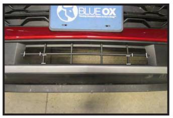
27. Using a reciprocating saw, trim the indicated area between the white marks to allow clearance for the attachment tabs and convenience links.
