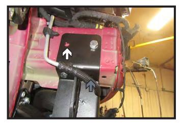
17. Using a 1/2" drill bit, drill the back side hole (white). Then using a 3/8" drill bit, drill the front bottom hole using the baseplate as a template (gray).
