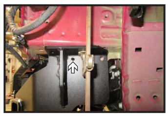
20. Using a 3/8" drill bit, drill the front side hole. Install 3/8" bolt with lock washer, flat washer and lock nut. Fully tighten driver side bolt and the four (4) front bolts on the passenger side of the vehicle. Remove vise grip.
