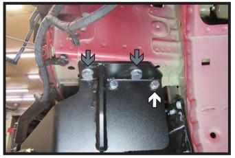
21. Using a 3/8" drill bit, drill the back side hole. Install 3/8" bolt with lock washer, flat washer and lock nut (white). Then using a 1/2" drill bit, drill the top two (2) holes using the baseplate as a template. Install 1/2" bolts with lock washer and whiz nut (gray).
