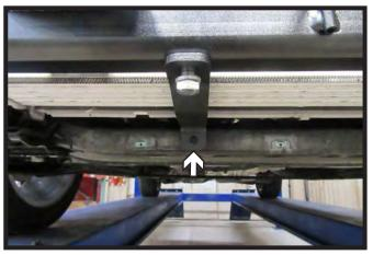
23. Ensure that the bracket is perpendicular and flush against the frame. Using a 1/2" drill bit, drill a hole in frame using the bracket as a template. Do this on both sides of the vehicle
