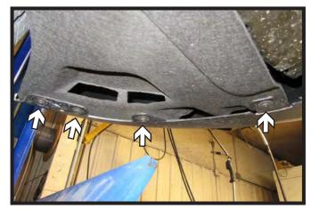
6. Using a T15 Torx, remove the four (4) bolts from the underside of the vehicle in front of the tire. Do this on both sides of the vehicle
