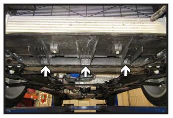
10. Using a 7MM socket, remove the five (5) bolts from the plastic shroud. There are two (2) bolts on top and three (3) bolts under the vehicle. Remove shroud and set aside to be reinstalled later.
