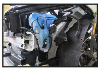
28. Reinstall the windshield washer fluid reservoir on the driver side of the vehicle. Reconnect all lines.
