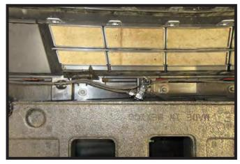
14. Remove the temperature sensor from the bracket on the back side of the fascia. Using a reciprocating saw, cut the bracket as shown. Relocate temperature sensor, connecting it to upper wire loom using the provided zip tie.
