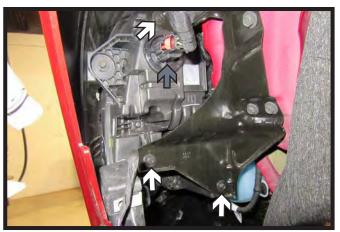
8. Pull back the wheel well liner. Using a 7MM socket, remove the three (3) bolts (white) attaching headlight housing to the frame. Unplug headlight (gray). Do this on both sides of the vehicle.
