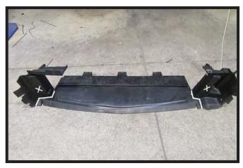
26. Using a reciprocating saw, remove the side pieces as indicated from the plastic shroud. Reinstall shroud using the bottom three (3) existing bolts.
