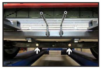
24. Install a 1/2" x 1-1/2" bolt with lock washer and whiz nut on each side. Tight all bracket bolts fully.
