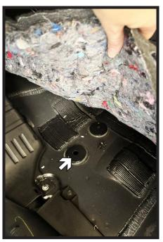
3. Using a 1/2" drill bit, drill a hole in the center of the plastic piece in the floor of the vehicle.
