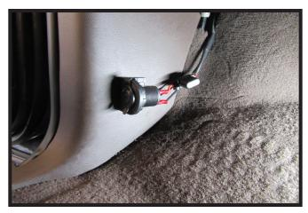
Reassemble plug and attach to mounting bracket. On the back of the 12V plug are positive (+) and negative (-) plugs. Connect the red wire to the positive (+) plug. Then connect the black wire to the negative (-) plug.
