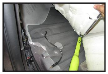
Run the unaltered end of the 14 GA wire through the hole towards the underside of the vehicle.
