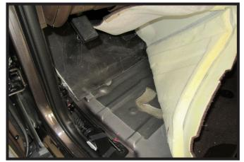
2. Pull up on the carpet. Locate the plastic piece that can be removed or drilled in the floor of the vehicle.
