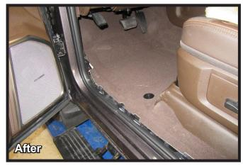
1. On the driver side of the vehicle, lift and pull up on the bottom and front door panel to unsnap and remove. Set panel(s) aside to be reinstalled later.
