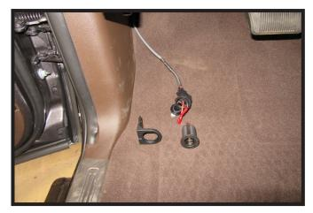
6. Disassemble plug from the mounting bracket.
