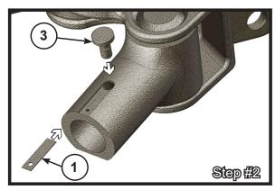
Insert the locking pin into the bar pivot hole. Stack two (2) springs on top of each other and slide the springs into the slot of the bar pivot until the springs seats into the groove of the locking pin and the rivet hole lines up with the holes in the springs.
