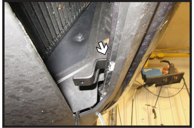
8b. Optional Breakaway: Using the existing bolt, attach the breakaway bracket to the gray clip as shown.
