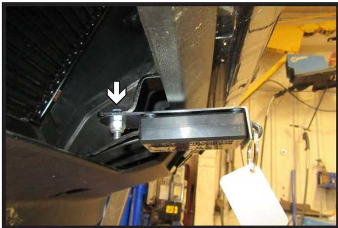
8c. Optional Breakaway: Attach breakaway switch to the breakaway bracket using the provided hardware.
