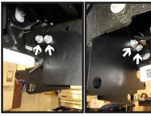
7. Attach the existing nuts to the four (4) bolts in baseplate side holes, two (2) on each side of the frame. Do this on both sides of the vehicle
