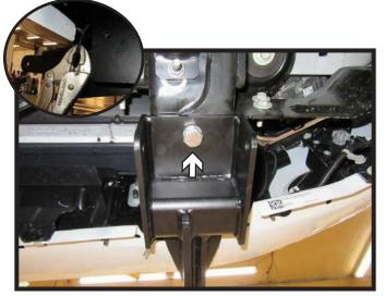
6. Install one (1) 5/8" bolt with lock washer and whiz flange nut into the bottom hole in the baseplate. Tighten. Do this on both sides of the vehicle.
