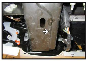
Sand down the indicated weld so that it is flush with the bottom of the frame with the hole to allow for a better baseplate installation. Spray sanded area with antirust paint. Do this on both sides of the vehicle.
