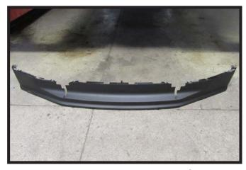
8. Hold the bumper valance as close to its original position, mark and trim the valance for the convenience links and attachment tabs as shown. Do this on both sides of the bumper valance.
