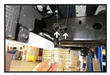
4. Feed lead wires through holes on both the of the frame. Place existing plate on the existing bolts and then attach lead wire to end of the dual bolts. Let bolts hang. Do this on both sides of the vehicle.
