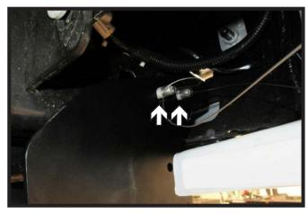
5. Raise baseplate into place and pull bolts through the frame so that the plate is flush against the inside of the frame and bolts are positioned horizontally. Do this on both sides of the vehicle.
