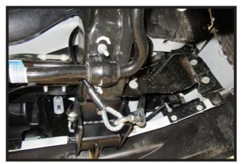
9. Attach the permanent baseplate safety cables to the provided convenience link on the baseplate. The photo above shows the recommended installation of the cables to frame of vehicle. Additional options may interfere with suggested mounting; in this case, secure the cables to a solid piece of the frame as described in the General Information sheet. Be sure the safety cables do not rub against any hoses or moving parts. Do this on **BOTH** sides of the vehicle.
