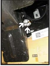
2. **Non-Tremor Models**: Using an 18MM socket, remove the four (4) bolts from the bracket below the tow hook housing. Remove bracket and set aside, it will not be reinstalled. Do this on both sides of the vehicle. Bolts and hardware will be used for the baseplate installation.
