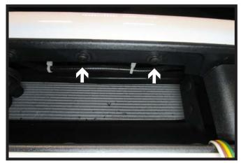
11. Remove the two (2) push pins from the grille opening. Attach the electrical bracket with the two (2) provided 1/4" screws.
