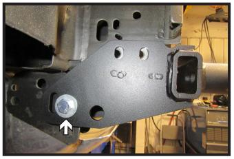
14. Raise the baseplate into position. Start a 1/2" x 5" bolt with flat washers, spacer tube, and nylon nut into forward back hole. Rotate baseplate up to ensure that the frame has been trimmed enough and the holes line up with existing holes on the frame. Leave loose. Do this on both sides of the vehicle.
