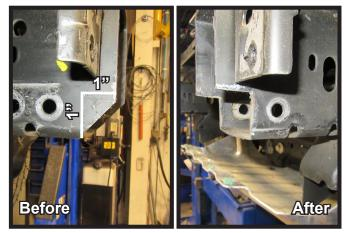
13. Measure 1" from the bottom of the frame edge and draw line then draw a 1" straight line across as shown. Using a reciprocating saw trim the marked area on both sides of the frame. Do this on both sides of the vehicle.
