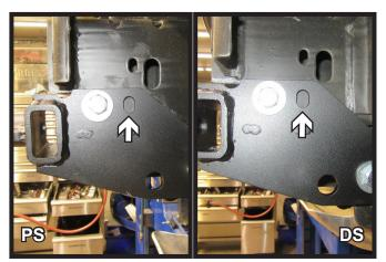
19. Using a 1/2" drill bit, drill out the top back hole in the frame using the baseplate as a template. Do this on both sides of the vehicle.
