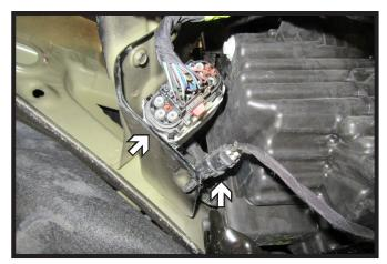
As the fascia is removed, unplug the two (2) electrical connections on the passenger side of the vehicle. Remove fascia and set aside to be reinstalled later.
