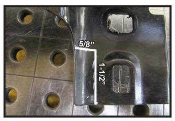
24. On the passenger side of the bumper a measure 5/8" x 1-1/2" area as shown. Using a reciprocating saw trim the indicated area.
