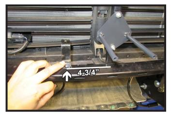
23. **Optional**: Measure 4-3/4" from the center and mark. Using a 1/4" drill bit, drill a hole in the cross member. Install breakaway bracket using the provided 1/4" bolt with hardware.
