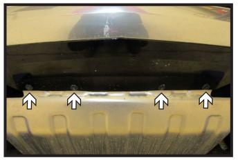
6. Using a 7MM socket, remove the four (4) bolts from the bottom of the fascia.
