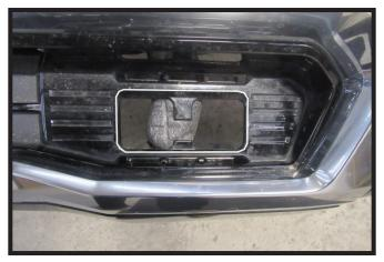
26a. **Chevy Models**: Using a reciprocating saw, trim the tow hook opening on the fascia as shown. Do this on both sides of the vehicle.
