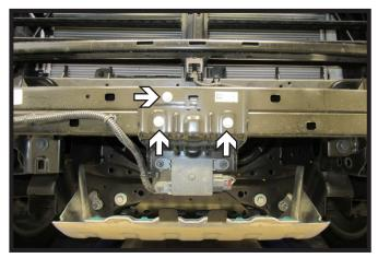
Using a 10MM socket, remove the three
