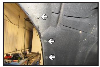
3a. **Chevy Models**: Using a T15 Torx, remove the six (6) bolts from the wheel well edge. Do this on both sides of the vehicle.
