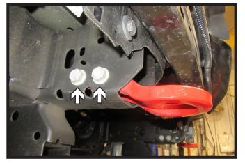
9. Using am 18MM socket and wrench, remove the two (2) bolts from the tow hook. Set tow hook aside, it will not be reinstalled. Do this on both sides of the vehicle.
