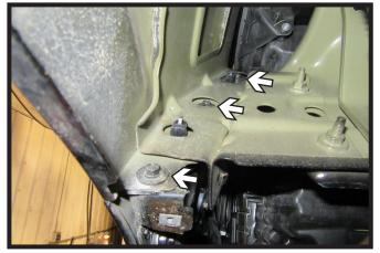
Pull back the wheel well liner. Using a 7MM socket, remove the three (3) bolts from the fascia joint. Do this on both sides of the vehicle.
