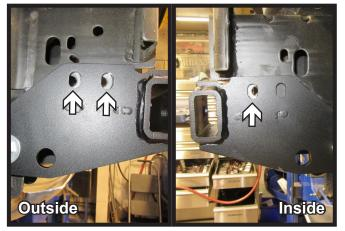
17. Using a 1/2" drill bit, ream out the existing holes as needed on both sides of the vehicle.
