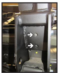
15. Ensure baseplate is flat flush with the bottom of the frame. Using a 1/2" drill bit, drill out the two (2) holes in the bottom of the frame using the baseplate at a template. Do this on both sides of the vehicle.
