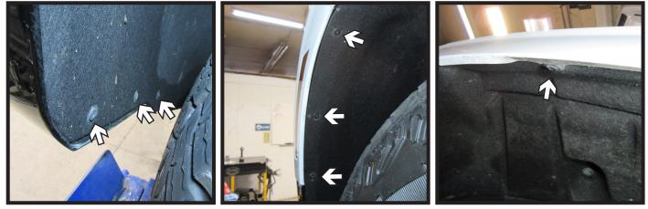
3b. **GMC Models**: Using a T15 Torx, remove the seven (7) bolts from the wheel well edge. Do this on both sides of the vehicle.
