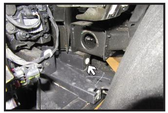
5b. GMC Models: Pull back wheel well liner. Using a 10MM socket, remove the one (1) bolt behind the fascia in front of the tire. Do this on both sides of the vehicle.
