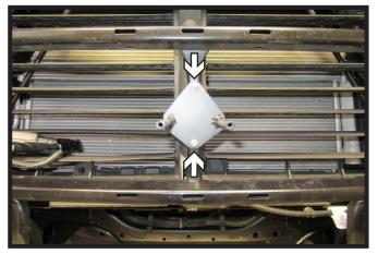
22. Mount the electrical bracket to the top center support brace using the two (2) provide 1/4" bolts with hardware.
