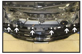
2. Using a 10MM socket, remove the six (6) bolts from the top of the fascia.
