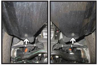
7. **GMC Models**: Using a 7MM socket, remove the two (2) bolts, one (1) on each side, from the bottom of the fascia next to the tires.
