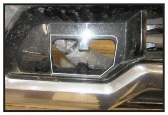
26b. **GMC Models**: Using a reciprocating saw, trim the tow hook opening on the fascia as shown. Do this on both sides of the vehicle.
