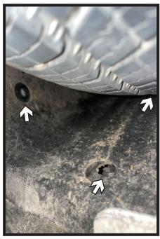
Using an 8MM socket, remove the three
