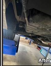
13. Flatten tab on the ground wire connector. Then reinstall ground wire to the original position on the driver side of the vehicle.
