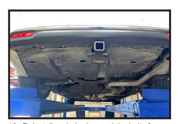
16. Reinstall underbody panel the bolts from secondary panel.
