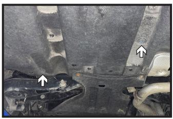
Using a phillips screw driver, remove the two (2) plastic plugs from the underbody panel.
