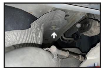
7. Using a 10MM socket, remove the two (2) nuts from the heat shield on the passenger side of the vehicle. Set heat shield aside, it will not be reinstalled.
