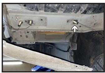
10. Place 1" x 3" spacer plate onto the lead wire then attach lead wire to the end of the 1/2" carriage bolt. Feed bolt then plate through the access hole. Ensure spacer plate is sitting flush against inner frame and the bolt is hanging vertically. Do this on both sides of the vehicle.
