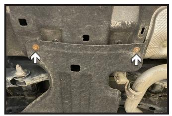
2. Using a 10MM socket, remove the two (2) bolts from the secondary panel, let panel hang.
