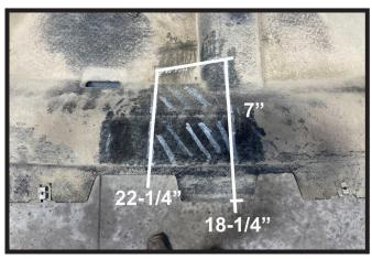
14. Measuring from the passenger side of the underbody panel, measure 18-1/4" to 22-1/4" from the edge and mark. Then measure 7" from the rear edge. Mark rectangle area as shown.
