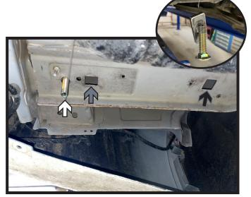
9. Starting with most rear hole in the frame (white), feed lead wire from the rear hole to the forward access hole in the frame (black). Place 1" x 2" spacer plate onto wire then attach lead wire to the end of the 1/2" carriage bolt (inset). Ensure spacer plate is sitting flush against inner frame and the bolt is hanging vertically. Repeat with second most rear hole (gray). Do this on both sides of the vehicle.
