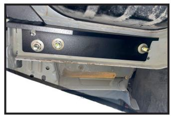
11. Raise the receiver hitch into place feeding the lead wires through the corresponding holes in the receiver. Remove lead wires and loosely install a conical washer and hex nut onto each bolt. Ensure the teeth on the conical washers are towards the hitch. Do this on both sides of the vehicle. Tighten all bolts.
