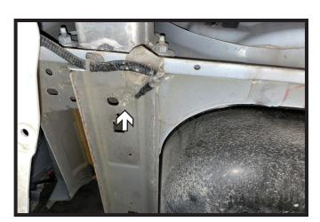
Using a 10MM socket, remove the nut attaching the ground wire to the frame on the driver side of the vehicle. It will be reinstalled later.
