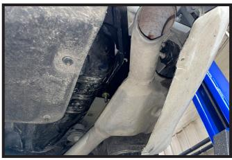
12. Raise the exhaust back into place and reinstall the rubber isolators.
