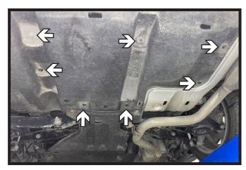
Using a 10MM socket, remove the seven(7) plastic nuts from the underbody panel.
