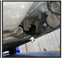
6. Support exhaust using a jack or stand. Remove the three (3) rubber isolators from the exhaust rods, one (1) in the center of the vehicle and two (2) on the passenger side. Lower exhaust to allow receiver hitch installation.
