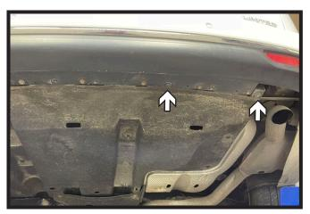
1. Using an 8MM socket, remove the six to eight (6-8) bolts from the underbody panel.
