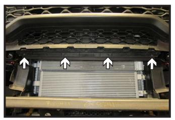
12. Remove the four (4) push pins from rubber piece below grille and remove. It will not be reinstalled.
