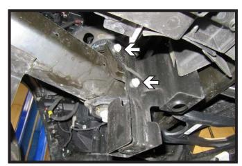
RHO Models: Using a 13MM socket, remove the two (2) bolts from the belly pan bracket. Remove bracket and set aside to be reinstalled later. Do this on both sides of the vehicle.
