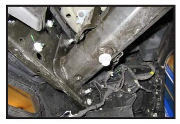
8. **Trucks with Tow Hooks:** Remove rubber grommet (white) and metal piece (gray) from back tow hook bolt. Reinstall the tow hook bolt and hardware. Do this on both sides of the vehicle. **Note**: If unable to remove tow hook bolt, may need to use a rubber mallet and hit downward on bolt to loosen.
