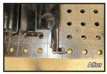
11. **RHO Models**: Using a reciprocating saw, cut along the weld at the bottom of the belly pan bracket. Remove piece from bracket. Do this on both brackets.
