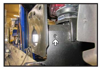
15. Using a 1/2" drill bit, drill the bottom hole and side hole in the frame using the baseplate as a template. Do this on both sides of the vehicle.
