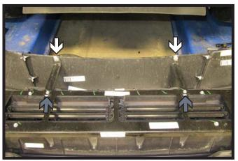
9. Using a T40 Torx remove the two (2) bolts (white) from the bottom of the brackets on the backside of the fascia. Then using a 10MM socket, remove the two (2) bolts (gray) from the top of the brackets. Remove brackets, they will not be reinstalled.
