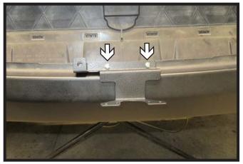
20. Install electrical bracket to the top of the bumper/fascia using the provided hardware.
