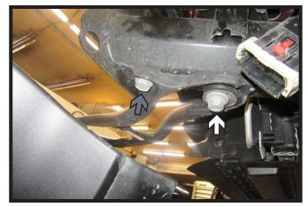
7. **Trucks with Tow Hooks:** Using a 21MM socket remove the front bolt (gray), and then using an 18MM socket remove the back bolt (white) attaching the tow hook to the frame. Remove tow hook. Do this on both sides of the vehicle. The tow hooks will not be reinstalled.
