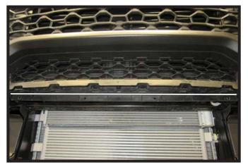
13. Using a reciprocating saw, cut a straight line (white line) across the plastic piece to remove the indicated area.
