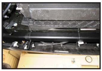
22. Reinstall bumper/fascia. Secure wire loom to the on the back of the fascia to the baseplate using the provided zip ties.
