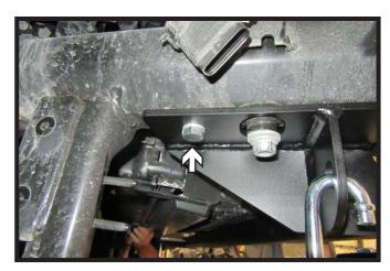
17. Install the 1/2" x 1-1/2" bolt with lock washer and whiz nut into the bottom back hole. Fully tighten all bolts at this time starting with the side bolt, then back bottom bolt, and finally the front bottom bolt. Do this on both sides of the vehicle.
