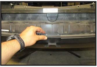
Hold electrical bracket on top of the bumper/fascia and mark holes. Using a 7/32" drill bit, drill two (2) holes.
