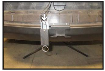
21. **Optional**: Attach breakaway switch to the electrical bracket using the provided hardware.
