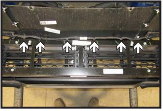
10. Remove the six (6) clips attaching the wire loom to the bottom of the shutter housing on the back of the bumper.
