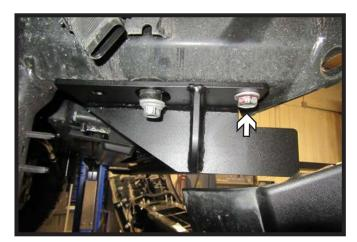
14. Raise baseplate into place and start the 14MM bolt with flat washer and nylon lock nut, hand tighten. Do this on both sides of the vehicle.
