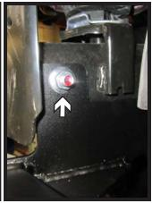
16. Place spacer plate onto 1/2" carriage bolt. Insert bolt and plate through access hole in the front of the vehicle frame. Install bolt and plate into side hole in baseplate and attach 1/2" flange whiz nut. Hand tighten. Do this on both sides of the vehicle.
