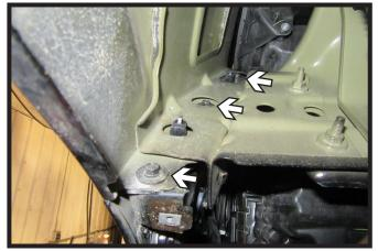
Pull back the wheel well liner. Using a 7MM socket, remove the three (3) bolts from the fascia joint. Do this on both sides
