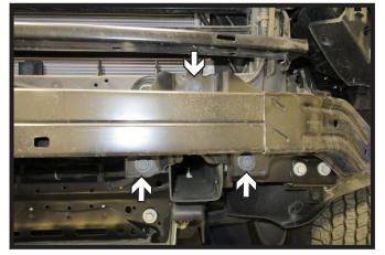
12. Using a 15MM socket, remove the six(6) bolts, three (3) on each side from the bumper. Remove bumper and set aside to be reinstalled later.
