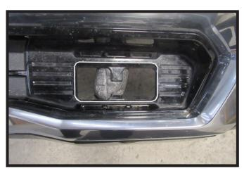
25. Using a reciprocating saw, trim the tow hook opening on the fascia as shown. Do this on both sides of the vehicle.
