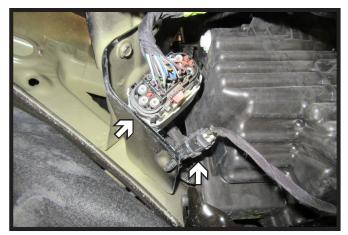
As the fascia is removed, unplug the two (2) electrical connections on the passenger side. Remove fascia and set aside to be reinstalled later.
