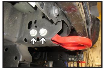
8. Using am 18MM socket and wrench, remove the two (2) bolts from the tow hook. Set tow hook aside, it will not be reinstalled. Do this on both sides of the vehicle.
