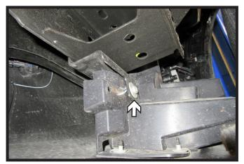
Using a 10MM socket, remove the one (1) bolt behind the fascia in front of the tire. Do this on both sides of the vehicle.
