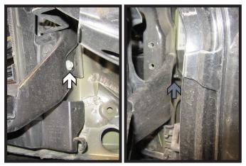
9. Using a 10MM socket, remove the bottom bolt (white) and loosen the top nut (gray) from the upper shutter housing. Do this on both sides of the vehicle.
