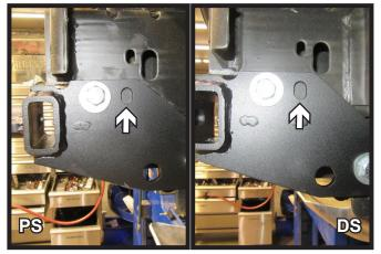
19. Using a 1/2" drill bit, drill out the hole top back hole in the frame using the baseplate as a template. Do this on both sides of the vehicle.
