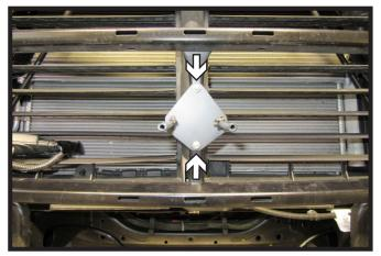
Mount the electrical bracket to the top center support brace using the two (2) provide 1/4" bolts with hardware.
