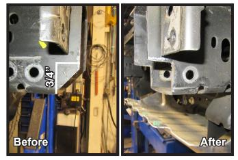
13. Measure 3/4" from the bottom of the frame edge and draw line then draw a straight line across as shown. Using a reciprocating saw trim the marked area on both sides of the frame. Do this on both sides of the vehicle.
