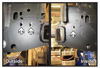
17. Using a 1/2" drill bit, ream out the existing holes on the passenger side of the vehicle.
