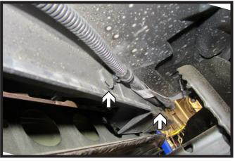
10. Remove the five (5) push pins from the bottom of the plastic shroud above the bumper. Unclip wire loom from the bottom of the shroud. Remove shroud and set aside to be reinstalled later.
