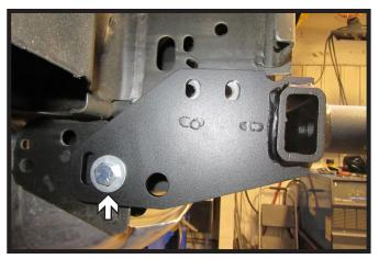
14. Slide baseplate onto vehicle. Start a 5/8" bolt with flat washers, spacer tube, and nylon nut into forward back hole. Rotate baseplate up to ensure that the frame has been trimmed enough and the holes line up with existing holes on the frame. Leave loose.
