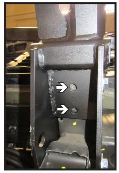
15. Ensure baseplate is flat flush with the bottom of the frame. Using a 1/2" drill bit, drill out the two (2) holes in the bottom of the frame using the baseplate at a template.
