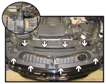
1. Remove the nine (9) push pins (white) from the fascia cover. Then using a T15 Torx, remove the two (2) screws from the hood latch handle (inset gray). Set aside the facia cover and hood latch handle to be re-installed later.
