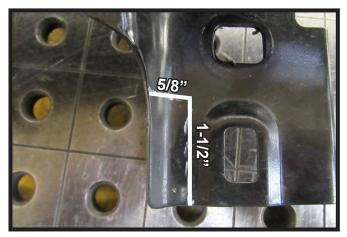
24. On the passenger side of the bumper a measure 5/8" x 1-1/2" area as shown. Using a reciprocating saw trim the indicated area. Reinstall bumper and reattach the ACC bracket and wire loom to the bumper. Reinstall plastic shroud above the bumper and reconnect wire loom.
