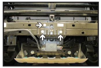
Using a 10MM socket, remove the three
