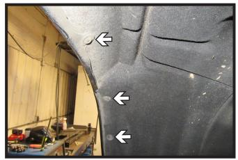
3. Using a T15 Torx, remove the six (6) bolts from the wheel well edge. Do this on both sides of the vehicle.
