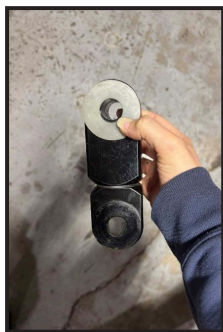
4. Place two (2) of the existing washers onto one side of the pivot block.
