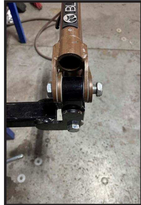
14. Insert 3/4" x 3-1/2" bolt with nut and tighten.
