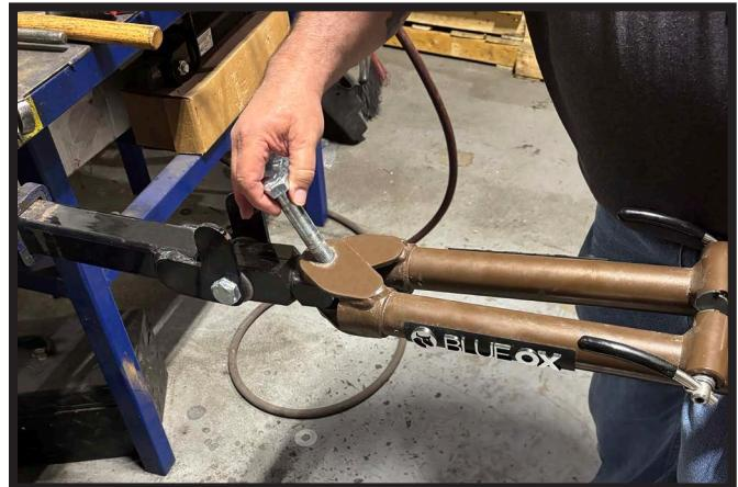
1. Place tow bar in a stored position. Using a 1-1/8" socket and wrench, remove the one (1) 3/4" nut attaching the tow bar legs.
