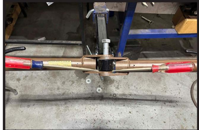
10. Insert the flat screwdrivers into the space that does not contain a washer. Tap on the end of the screwdrivers with rubber mallet to create a gap for the washers to be inserted.
