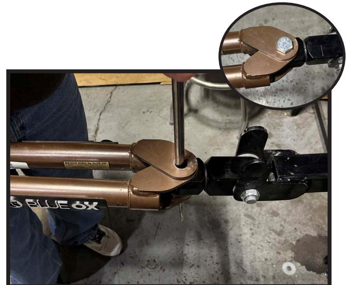
8. Using the alignment tool, align all of the holes on the tow bar. Insert 3/4" x 3-1/2" bolt through aligned holes (inset).
