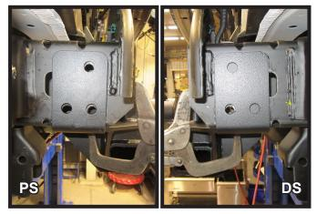
14. Slide the baseplate onto the vehicle and line up the holes of the baseplate as closely as possible to the existing holes in the frame. Clamp in place using large vise grips.
