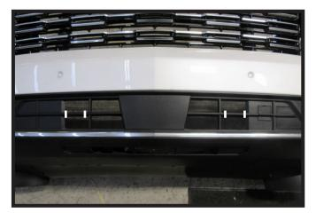
21. Using a reciprocating saw, trim the indicated areas of the fascia to allow clearance for the attachment tabs and convenience links.
