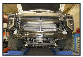
20. Reinstall bottom bolts and tighten upper nuts on top shutter housing.
