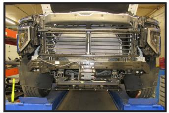
Reinstall bumper. Reattach the ACC bracket and wire loom(s) to the bumper.
