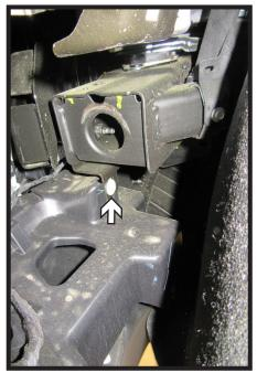
5. Pull back the wheel well liner. Using a 10MM socket, remove the one (1) bolt behind the fascia in front of the tire. Do this on both sides of the vehicle.
