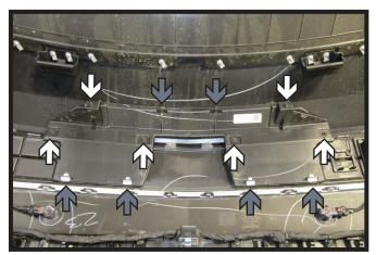
9. **Gas Models**: Using a 7MM socket, remove the six (6) bolts (white) from the cover on the back side of the fascia. Then remove the six (6) clips (gray). Remove cover from back of fascia, it will not be reinstalled.
