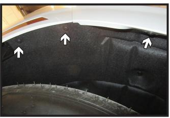
3. Using a T15 Torx, remove the six (6) bolts from the wheel well edge. Do this on both sides of the vehicle.
