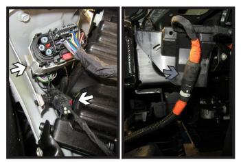
7b. Diesel Models: As the fascia is removed, unplug the two (2) electrical connections on the passenger side (white) and one (1) electrical connection on the driver side (gray). Remove fascia and set aside to be reinstalled later.
