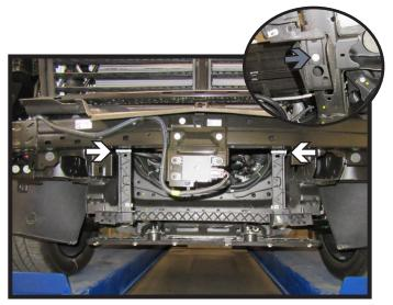
Gas Models: Using a reciprocating saw, cut the top of the plastic piece on each side as indicated. Then using a 10MM socket, remove the two (2) bolts, one (1) on each side, from the bottom of the plastic piece (inset). Remove plastic piece, it will not be reinstalled.
