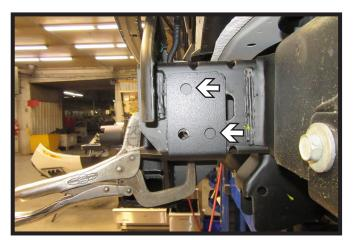
16. Using a 1/2" drill bit, drill out the driver side holes in the frame using the baseplate as a template. Then ream out the existing holes on both side of the vehicle using a 1/2" drill bit.
