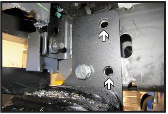
12. Using a 1/2" drill bit, drill the remaining two (2) side holes on the passenger side of the vehicle using the baseplate as a template. Insert two (2) 1/2" bolts with lock washers and whiz nuts. Tighten all side bolts at this time.
