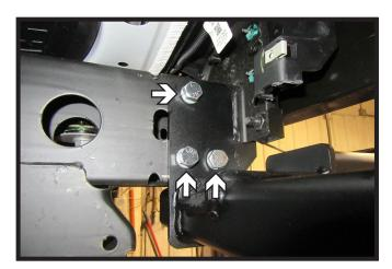
11a. Slide baseplate onto the vehicle and insert three (3) 1/2" bolts with lock washers and whiz nuts into side holes on the driver side of the vehicle. Hand tighten.
