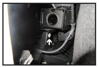
Pull back the wheel well liner. Using a 10MM socket, remove the one (1) bolt behind the fascia in front of the tire. Do this on both sides of the vehicle.
