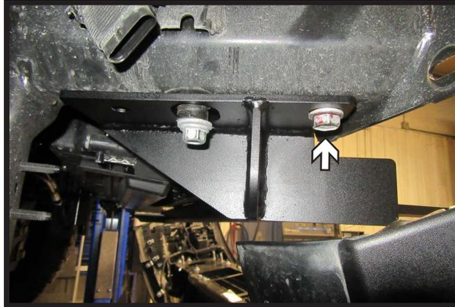
6. Raise baseplate into place and start the 14MM bolt with flat washer and nylon lock nut, hand tighten. Do this on both sides of the vehicle.
