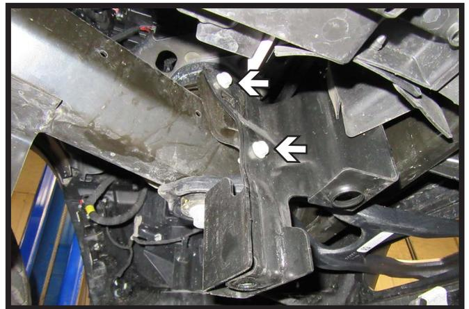
3. **RHO Models:** Using a 13MM socket, remove the two (2) bolts from the belly pan bracket. Remove bracket and set aside to be reinstalled later. Do this on both sides of the vehicle.
