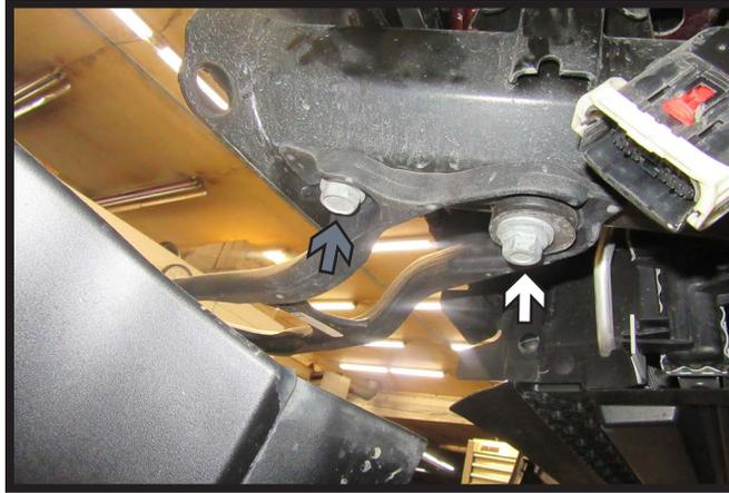
1. **Trucks with Tow Hooks:** Using a 21MM socket remove the front bolt (gray), and then using an 18MM socket remove the back bolt (white) attaching the tow hook to the frame. Remove tow hook. Do this on both sides of the vehicle. The tow hooks will not be reinstalled.
