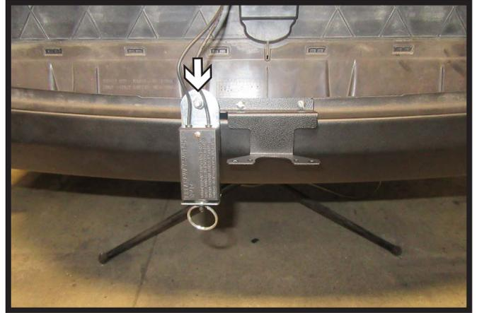
13. **Rebel/RHO Models (Optional):** Attach breakaway switch to the electrical bracket using the provided hardware.
