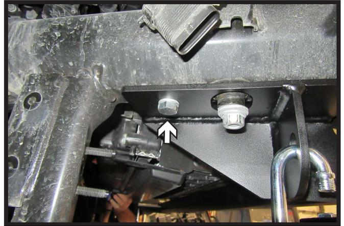
9. Install the 1/2" x 1-1/2" bolt with lock washer and whiz nut into the bottom back hole. Fully tighten all bolts at this time starting with the side bolt, then back bottom bolt, and finally the front bottom bolt. Do this on both sides of the vehicle.
