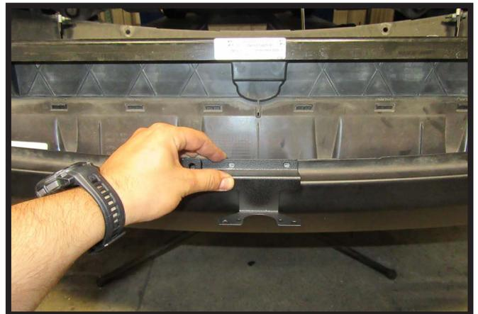
11. **Rebel/RHO Models:** Hold electrical bracket on top of the bumper/fascia and mark holes. Using a 7/32" drill bit, drill two (2) holes.
