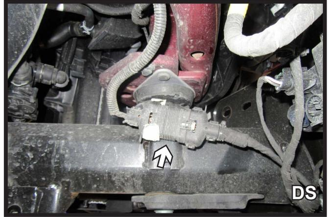
4. Unplug the one (1) electrical connection on each side of the vehicle.
