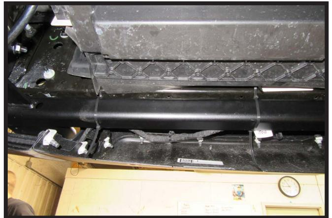
14b. **Rebel/RHO Models:** Reinstall bumper/fascia. Secure wire loom to the on the back of the fascia to the baseplate using the provided zip ties.
