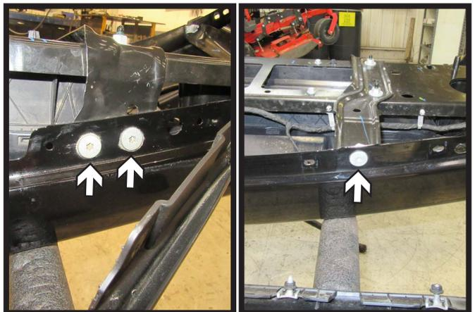
6. Pull back rubber piece. Using a T40 Torx, remove the three (3) bolts from the bumper. There are two (2) on the top and one (1) on the bottom. Do this on both sides of the bumper.
