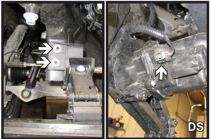
10. Using a 13MM socket, remove the two (2) nuts from the automatic valence. Do this on both sides of the vehicle. Unplug the electrical connection on the driver side and remove valence and set aside to be reinstalled later.
