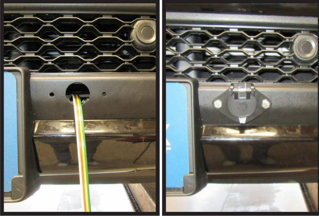
15. **Non-Rebel/RHO Models:** Using a 1-1/2" hole saw drill a hole in the bumper on the driver side for the electrical plug as shown. Hold plug in place, using a 1/4" drill bit, drill the two (2) holes in the bumper for the bolts using the plug as a template. Install plug using provided hardware.
