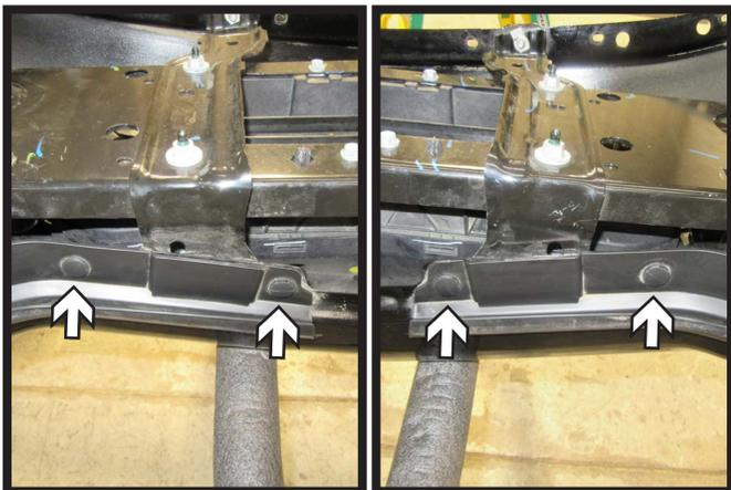
5. Remove the four (4) push pins, two (2) on each side, from the rubber piece on the top of the bumper.
