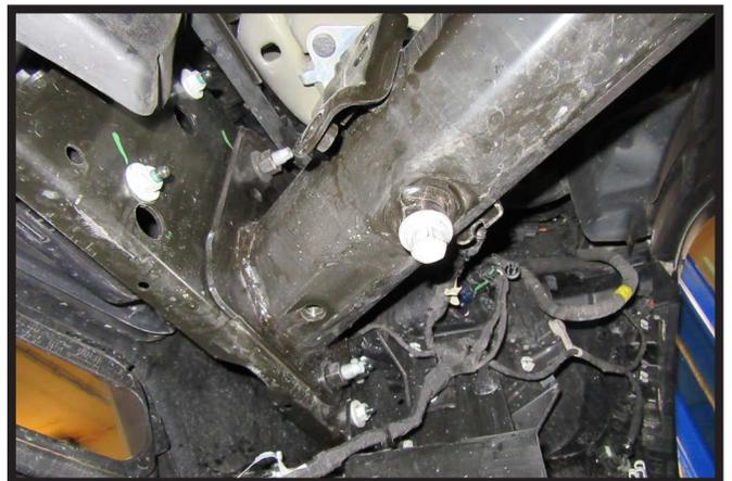
2. **Trucks with Tow Hooks:** Remove rubber grommet (white) and metal piece (gray) from back tow hook bolt. Reinstall the tow hook bolt and hardware. Do this on both sides of the vehicle. **Note:** If unable to remove tow hook bolt, may need to use a rubber mallet and hit downward on bolt to loosen.
