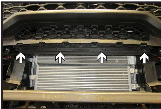
4. Remove the four (4) push pins from rubber piece below grille and remove. It will not be reinstalled.
