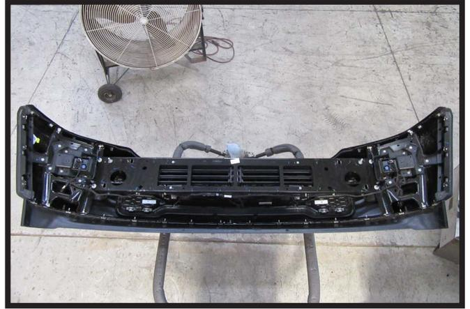
8. Reinstall the four (4) push pins on the top of the bumper and the bumper valence to the bottom of the bumper.
