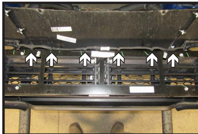
8. Remove the six (6) clips attaching the wire loom to the bottom of the shutter housing on the back of the bumper.
