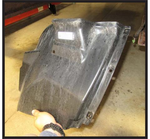
1. Using an 8MM socket, remove the five (5) bolts from the wheel well. Remove plastic piece and set aside to be reinstalled later. Do this on both sides of the vehicle.
