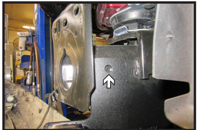
7. Using a 1/2" drill bit, drill the bottom hole and side hole in the frame using the baseplate as a template. Do this on both sides of the vehicle.
