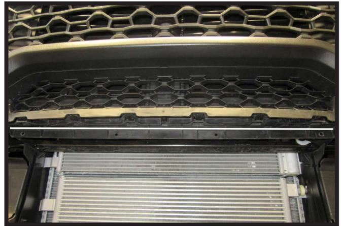
5. Using a reciprocating saw, cut a straight line (white line) across the plastic piece to remove the indicated area.
