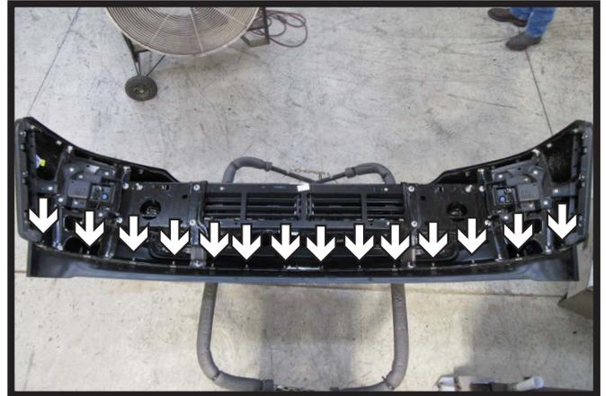
4. Using a 10MM socket, remove the fourteen (14) nuts from the bottom of the bumper. Remove bumper valence and set aside to be reinstalled later.
