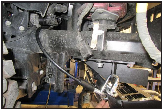
10. Attach the permanent baseplate safety cables to the provided convenience link on the baseplate. The photo above shows the recommended installation of the cables to frame of vehicle. Additional options may interfere with suggested mounting; in this case, secure the cables to a solid piece of the frame as described in the General Information sheet. Be sure the safety cables do not rub against any hoses or moving parts. Do this on **BOTH** sides of the vehicle.
