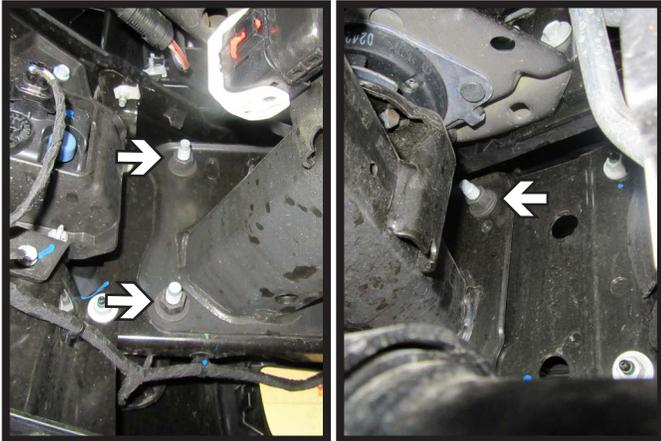
3. Using an 18MM socket, remove the three (3) bolts from the back of the bumper. Do this on both sides of the vehicle. Remove bumper and set aside to be reinstalled later.
