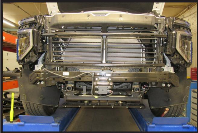
18. Reinstall bumper. Reattach the ACC bracket and wire loom to the bumper.
