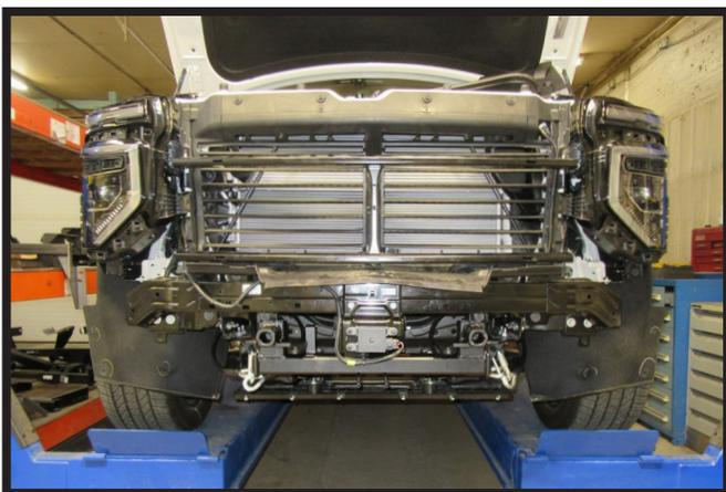
20. Reinstall plastic shroud above the bumper and reconnect wire loom.
