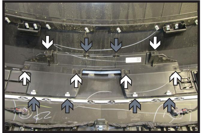
9. Using a 7MM socket, remove the six (6) bolts (white) from the cover on the back side of the fascia. Then remove the six (6) clips (gray). Remove cover from back of fascia, it will not be reinstalled.
