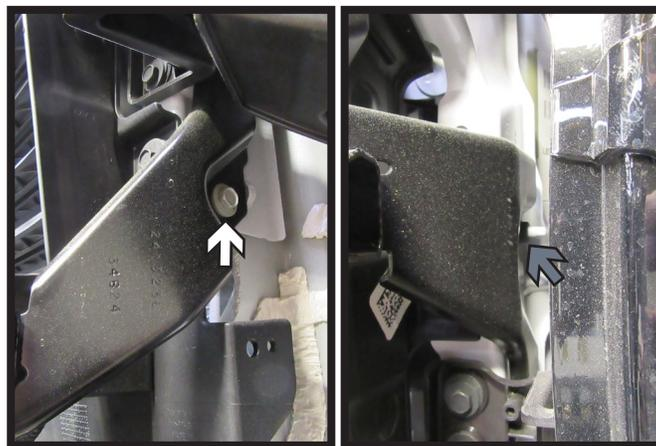
10. Using a 10MM socket, remove the bottom bolt (white) and loosen the top nut (gray) from the upper shutter housing. Do this on both sides of the vehicle.
