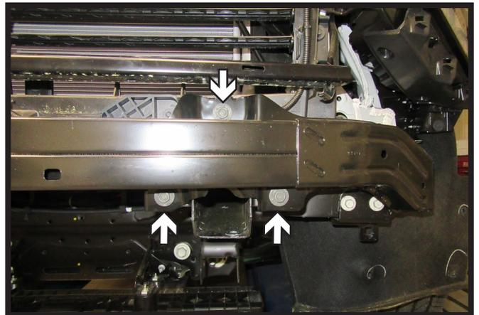
12. Using a 10MM socket, remove the three (3) bolts attaching the adaptive cruise control (ACC) bracket to the bumper. Unclip wire loom from the bumper. Set ACC sensor with bracket out of the way for baseplate installation.
