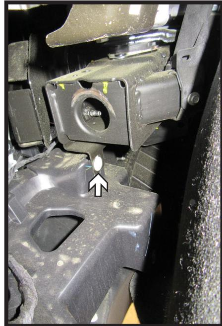
5. Pull back the wheel well liner. Using a 10MM socket, remove the one (1) bolt behind the fascia in front of the tire. Do this on both sides of the vehicle.
