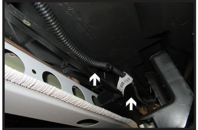
11. Remove the five (5) push pins from the bottom of the plastic shroud above the bumper. Unclip wire loom from the bottom of the shroud. Remove shroud and set aside to be reinstalled later.
