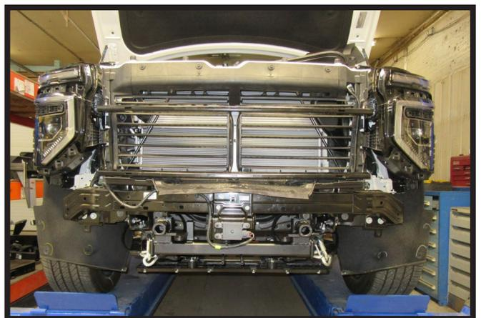
21. Reinstall bottom bolts and tighten upper nuts on top shutter housing.
