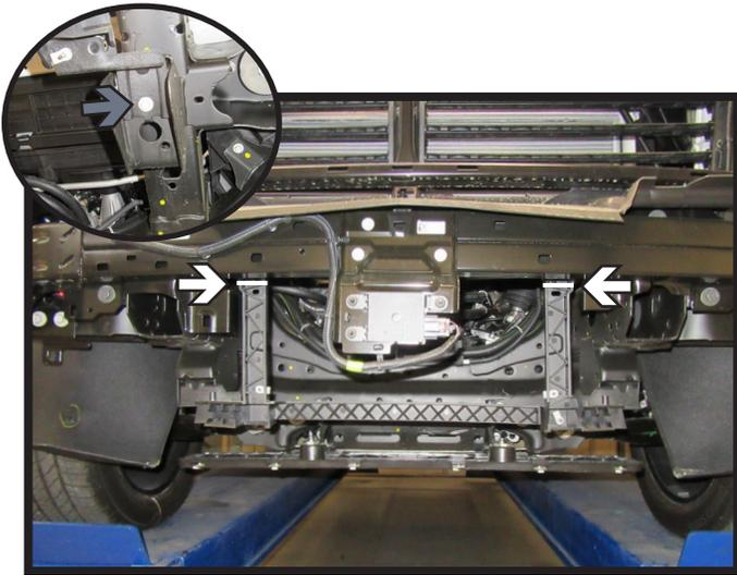
8. Using a reciprocating saw, cut the top of the plastic piece on each side as indicated. Then using a 10MM socket, remove the two (2) bolts, one (1) on each side, from the bottom of the plastic piece (inset). Remove plastic piece, it will not be reinstalled.
