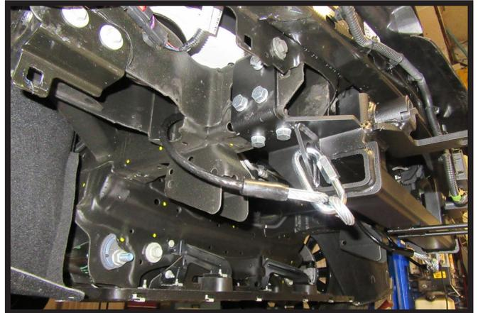
19. Attach the permanent baseplate safety cables to the provided convenience link on the baseplate. The photo above shows the recommended installation of the cables to frame of vehicle. Additional options may interfere with suggested mounting; in this case, secure the cables to a solid piece of the frame as described in the General Information sheet. Be sure the safety cables do not rub against any hoses or moving parts. Do this on **BOTH** sides of the vehicle.
