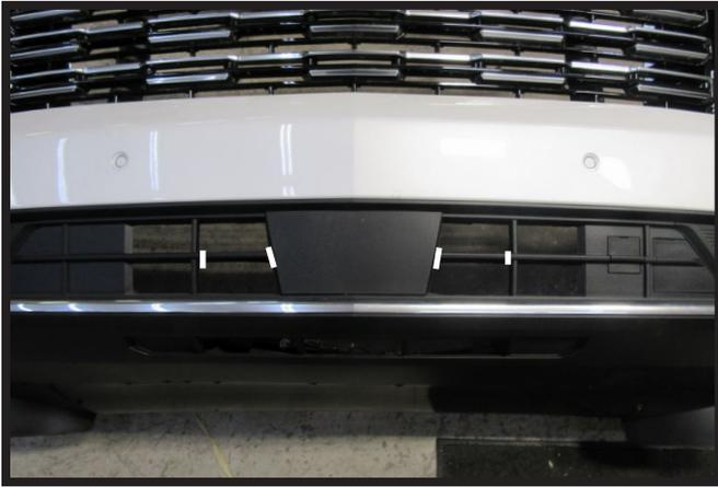
22. Using a reciprocating saw, trim the indicated areas of the fascia to allow clearance for the attachment tabs and convenience links.
