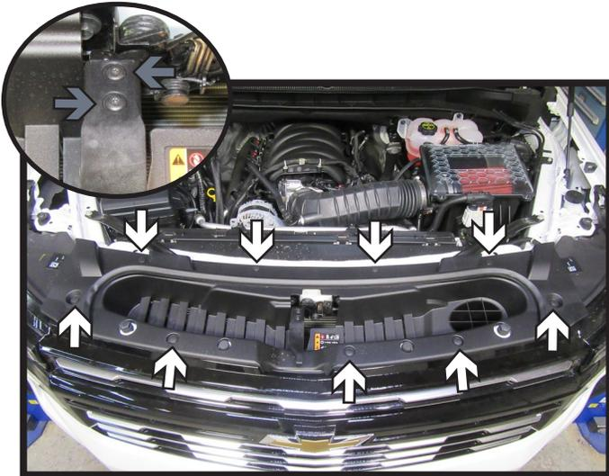
1. Remove the nine (9) push pins (white) from the fascia cover. Then using a T15 Torx, remove the two (2) screws from the hood latch handle (inset gray). Set aside the fascia cover and hood latch handle to be re-installed later.
