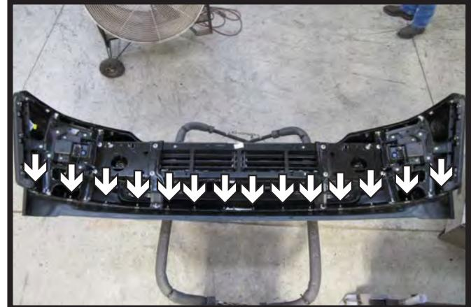
3. Using an 18MM socket, remove the three (3) bolts from the back of the bumper. Do this on both sides of the vehicle. Remove bumper and set aside to be reinstalled later.
