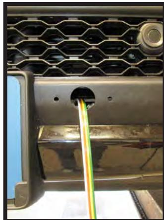
**15. Non-Rebel/RHO Models:** Using a 1-1/2" hole saw drill a hole in the bumper on the driver side for the electrical plug as shown. Hold plug in place, using a 1/4" drill bit, drill the two (2) holes in the bumper for the bolts using the plug as a template. Install plug using provided hardware.
