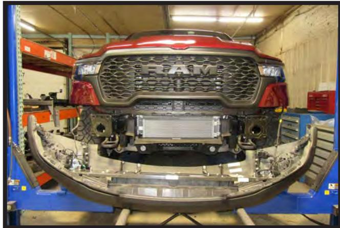
6. Remove bumper but do not disconnect upper electrical connection on each side. Place bumper out of the way for baseplate installation on a stand or other safe option.
