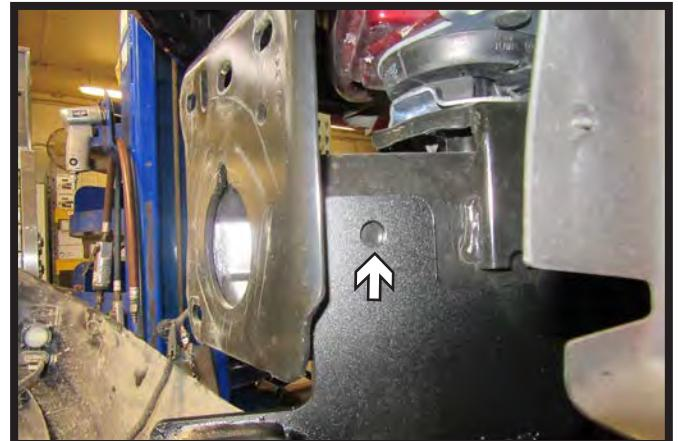
7. Using a 1/2" drill bit, drill the bottom hole and side hole in the frame using the baseplate as a template. Do this on both sides of the vehicle.
