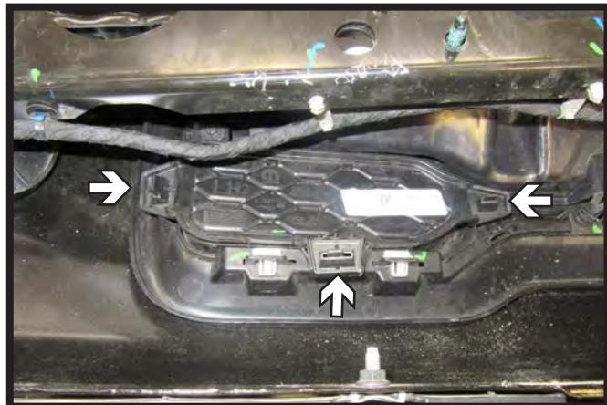
9. **Vehicles without Tow Hooks:** Unclip the three (3) clips from the tow hook cover and push towards the back of the bumper to remove. Do this on both sides of the bumper.
