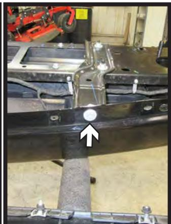
5. Remove the four (4) push pins, two (2) on each side, from the rubber piece on the top of the bumper.
