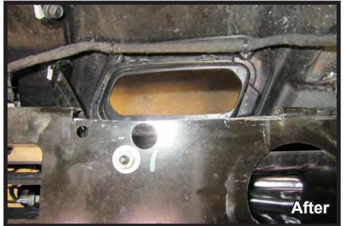
12. In necessary, use a reciprocating saw to trim the indicated area from the metal piece on the back of the bumper as shown. Do this on both sides of the vehicle.
