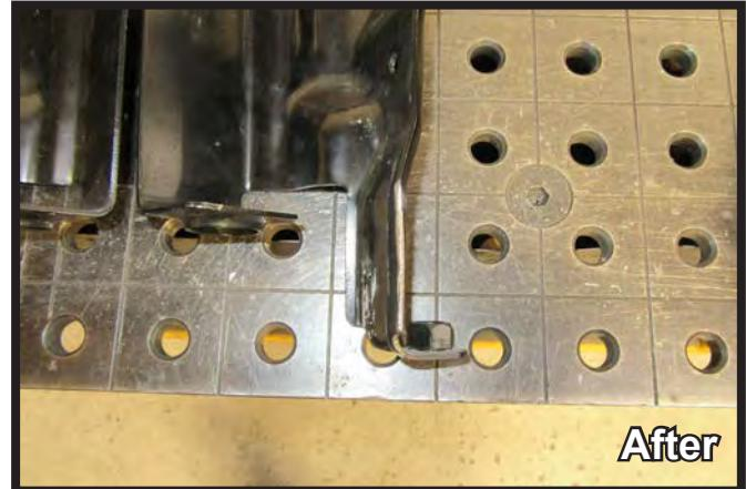
3. **RHO Models:** Using a reciprocating saw, cut along the weld at the bottom of the belly pan bracket. Remove piece from bracket. Do this on both brackets.
