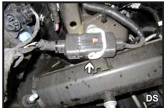
2. Unplug the one (1) electrical connection on each side of the vehicle.
