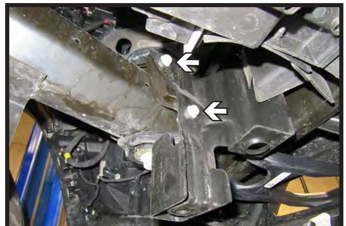
3. **RHO Models:** Using a 13MM socket, remove the two (2) bolts from the belly pan bracket. Remove bracket and set aside to be reinstalled later. Do this on both sides of the vehicle.
