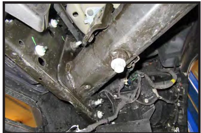
2. **Trucks with Tow Hooks:** Remove rubber grommet (white) and metal piece (gray) from back tow hook bolt. Reinstall the tow hook bolt and hardware. Do this on both sides of the vehicle.
