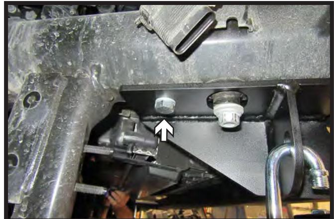
8. Place spacer plate onto 1/2" carriage bolt. Insert bolt and plate through access hole in the front of the vehicle frame. Install bolt and plate into side hole in baseplate and attach 1/2" flange whiz nut. Hand tighten. Do this on both sides of the vehicle.
