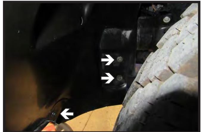
1. Using an 8MM socket, remove the five (5) bolts from the wheel well. Do this on both sides of the vehicle.
