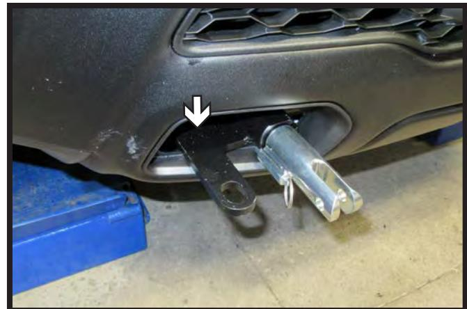
**16. Non-Rebel/RHO Models (Optional):** Attach breakaway switch to the hole in the convenience link using the provided hardware.
