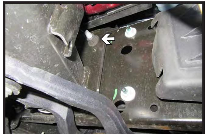
5. Using an 18MM socket, Remove the three (3) nuts from the back side of the bumper. Do this on both sides of the vehicle.
