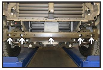
16. Using a 13MM socket, remove the five (5) bolts from the tube below the ACC sensor. Then remove the one (1) push pin attaching the wire loom to top of tube. Remove tube and set aside to be reinstalled later. Set sensor and wire loom out of the way for baseplate installation.
