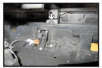
11. Remove the one (1) push pin from the center of the vehicle behind the grille.
