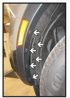
3. Remove the six (6) push pins from the wheel well. Do this on both sides of the vehicle.
