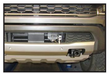
23. Install electrical bracket onto bumper at the top of the grille opening as shown using 1/4" bolts and hardware.
