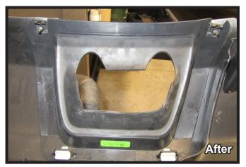
27. Using a utility knife, trim the tow hook opening as shown to allow clearance for the baseplate. Do this on both sides of the vehicle.
