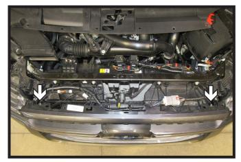
Using an 8MM socket, remove the two (2) bolts, one (1) on each side, from the bottom of the fascia.
