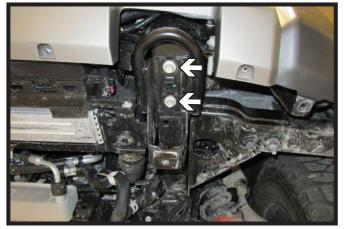
4. Using a 15MM socket, remove the two (2) bolts from the tow hook. Do this on both sides of the vehicle.
