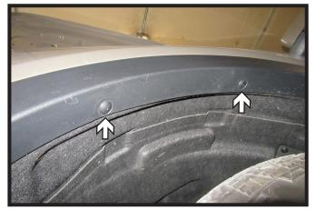
5. Using a Phillips screwdriver, remove the two (2) push pins from the top of the wheel well edge. Do this on both sides of the vehicle.
