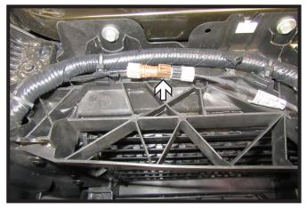
12. Unplug the electrical on the top of the vehicle and unclip the wire loom from the vehicle.
