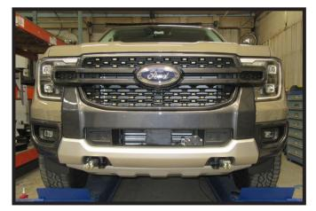
31. Reinstall fascia, fasica cover, and reconnect all electrical connections.
