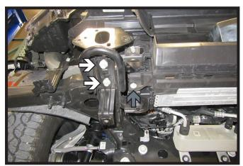
17. Using a 15MM socket, remove the two (2) bolts (white) from the bottom of the two hook. Then using an 8MM socket, remove the one (1) bolt (gray) next to the tow hook. Remove tow hook, it will not be reinstalled. Do this on both sides of the vehicle.
