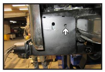
14. Using a 3/8" drill bit, drill out the rear hole on the side of the frame using the baseplate as a template. May need to ream out the front hole. Do this on both sides of the vehicle.
