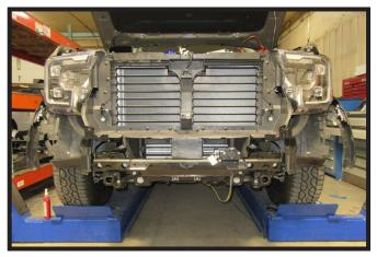
28. Reinstall tube and reattach ACC bracket to the tube. Reattach wire loom to the top of the tube.
