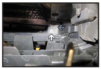
10. Using a 10MM socket and two (2) 10" socket extensions, remove the two (2) bolts (white) from behind the grill. There is one (1) on each side. Remove the two (2) push pins (gray), one (1) on each side, from behind the grille.
