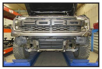
Remove bumper and set aside to be reinstalled later. Set ACC bracket and sensor on top of vehicle, out of the way for baseplate installation.
