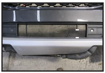
26. Using a reciprocating saw, trim the vertical slat on the driver side of the vehicle as shown to allow clearance for the electrical bracket.
