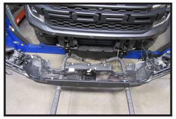
20. Support bumper in front of vehicle. Reinstall the ACC bracket. Reconnect the electrical connections on each side of the bumper and reinstall wire loom.
