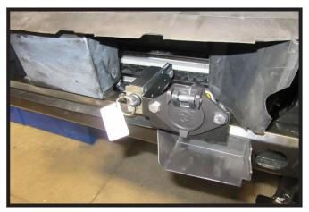
29. **Optional**: Install breakaway switch onto the electrical bracket as shown using provided hardware.
