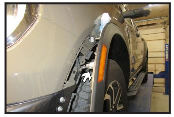
Pull back the wheel well trim, releasing the two (2) push pins, past the fascia joint. Disconnect the electrical connection. Prop trim away from the vehicle using a soft cloth. Do this on both sides of the vehicle.
