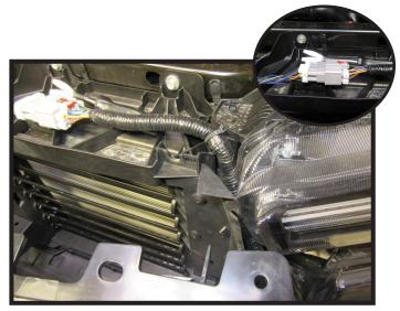
13. Unplug the electrical connection on the driver side of the vehicle (inset) and unclip wire loom from the vehicle. Remove fascia and set aside to be reinstalled later.
