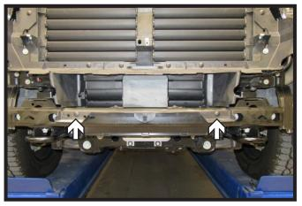
Using a Phillips screwdriver, remove the two (2) push pins from the plastic piece below the Adaptive Cruise Control (ACC).
