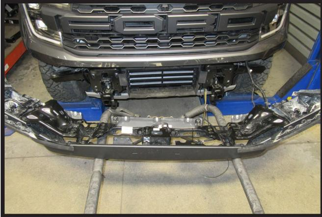
21 . Reinstall metal shields on each side of the back of the bumper. Reinstall remaining areas of the wire loom to shields.
