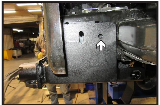
14. Using a 3/8" drill bit, drill out the rear hole on the side of the frame using the baseplate as a template. May need to ream out the front hole. Do this on both sides of the vehicle.
