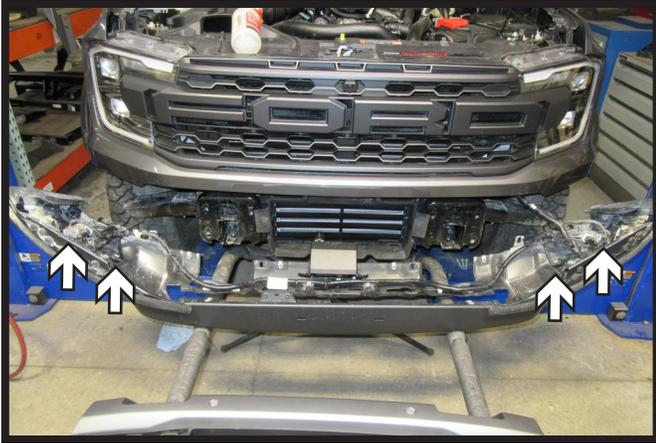
11. Disconnect the two (2) electrical connections on each side of the bumper. Unclip the rest of the wire loom from the back of the bumper.
