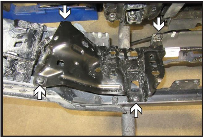
9. Unclip the wire loom from the metal shield on the backside of the bumper. Then using a T40 Torx, remove the four (4) bolts attaching the shield to the bumper. Remove shield and set aside to be reinstalled later. Do this on both sides of the vehicle.
