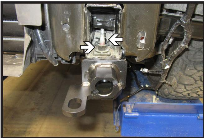
13. Slide baseplate onto vehicle. Reinstall the bottom two (2) existing bolts. As the bolts are tightened, push side plates towards the vehicle frame so the baseplate is flush against the frame. Do this on both sides of the vehicle.
