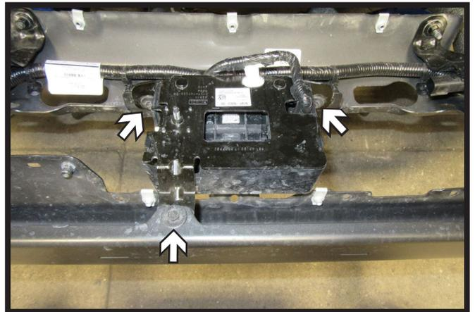
10. Using a 10MM socket, remove the three (3) bolts from the Adaptive Cruise Control (ACC) bracket. **Do Not unplug the ACC sensor.**
