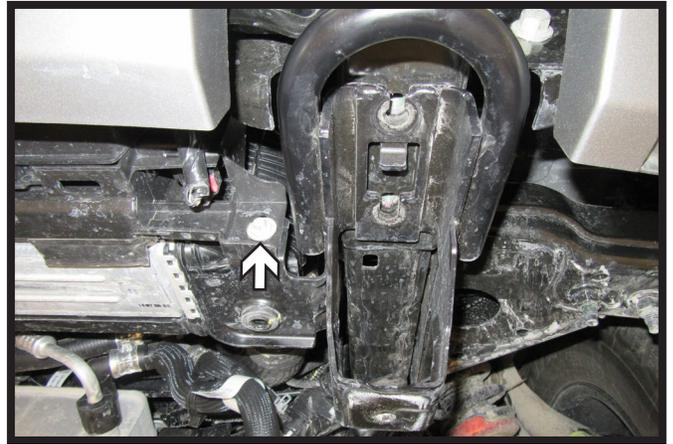
5. Using an 8MM socket, remove the one (1) bolt next to the tow hook. Remove tow hook, it will not be reinstalled. Do this on both sides of the vehicle.
