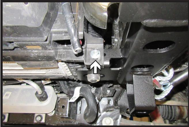
17. Starting from the rear of the vehicle, install the 1/4" bolt with flat washer and nut into hole attaching the bottom shutters to baseplate. Do this on both sides of the vehicle.
