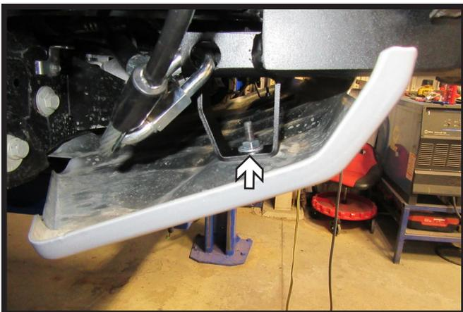
19. Reinstall skid plate using the two (2) existing bolts and provided flat washers and nuts.
