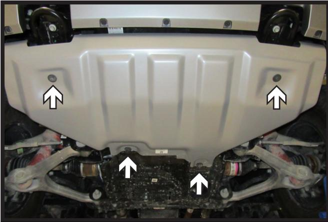
1. Using a 15MM socket, remove the four (4) bolts from the skid plate. Remove skid plate and set aside to be reinstalled later.
