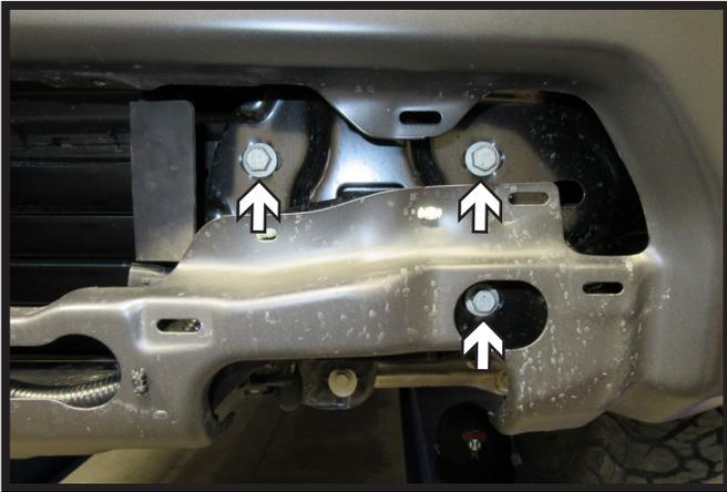
7. Using a 15MM socket, remove the three (3) bolts from the bumper bracket. Do this on both sides of the vehicle.
