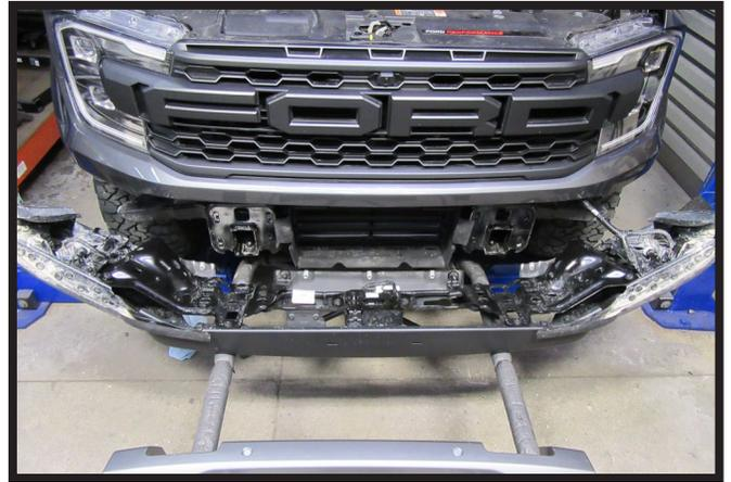
8. Remove the bumper, support and set in front of the vehicle. **Do not disconnect electrical.**
