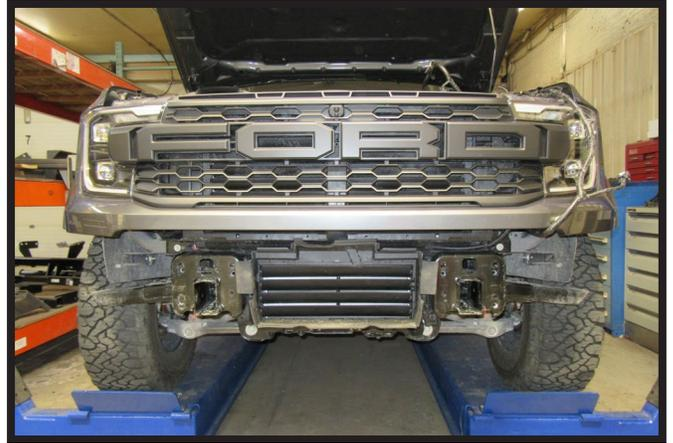
12. Remove bumper and set aside to be reinstalled later. Set ACC bracket and sensor on top of vehicle, out of the way for baseplate installation.
