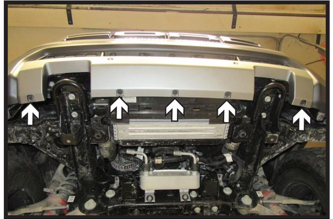
2. Using a 10MM socket, remove the five (5) bolts from the bottom of the fascia.
