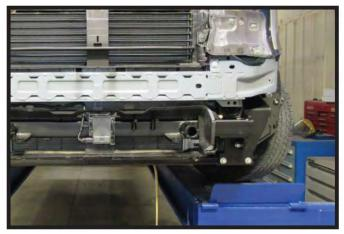
29. Reinstall the black box on the driver side of the vehicle. Reattach the wire loom to front of the box and to the bottom bolt on the backside. If the box touches the baseplate bolt head, bend back plate slightly to create clearance.
