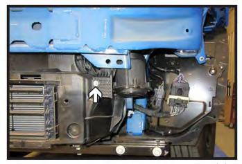
9. Using a 8MM socket, remove the one (1) bolt from the speaker mounting bracket on the driver side of the vehicle. Unplug electrical on the back of the speaker. Remove the pedestrian alert speaker and set aside to be reinstalled later.
