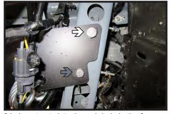
24. Insert nut plate through hole in the frame. Insert a 1/2" bolt into the top hole (white) and a 3/8" bolt into the bottom hole (gray). Bend frame piece back into place. Tighten all bolts. Do this on both sides of the vehicle.
