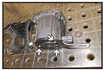
16. Using the existing bolts, attach the provided new mounting bracket to the bottom of the speaker as shown.
