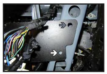
22. Using a 3/8" drill bit, drill out the back bottom hole (white) using the baseplate as a template. If needed use a 1/2" drill bit to ream out the back top hole (gray). Do this on both sides of the vehicle.
