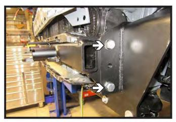
21. Slide the baseplate center piece into place. Install four (4) 1/2" bolts with nylon lock nuts, two (2) on each side. Ensure the center tube is level then tighten all bolts at this time.
