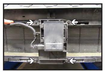
13. **Vehicles with ACC**: Using a T30 Torx, remove the four (4) bolts from the adaptive cruise control (ACC) mounting bracket. Set ACC bracket out of the way for installation.
