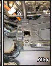
Using a reciprocating saw, carefully trim the indicated rib on top of the fascia and release clip. Do this on both sides of the vehicle.
