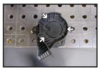
15. Using a T20 Torx, remove the three (3) bolts from the bottom of the pedestrian alert speaker. Remove the mounting bracket from the speaker.
