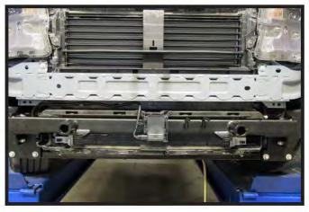
Vehicles with ACC: Reinstall the ACC mounting bracket.
