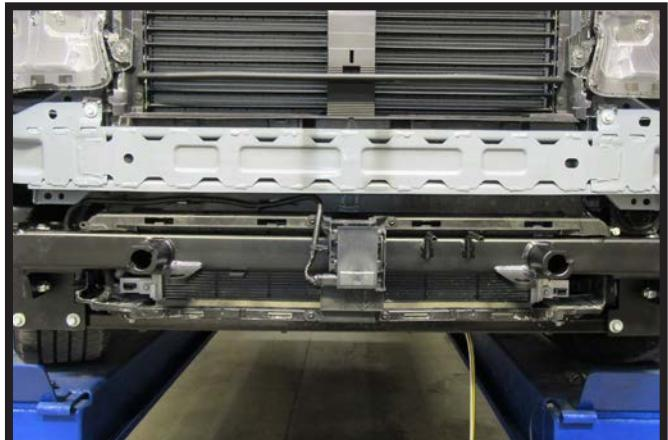
26. **Vehicles with ACC:** Reinstall the ACC mounting bracket.
