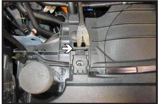
2. Using a flat head screw driver or similar tool, pull up on the plastic piece and outward on the fascia to release clip. Do this on both sides of the vehicle.
