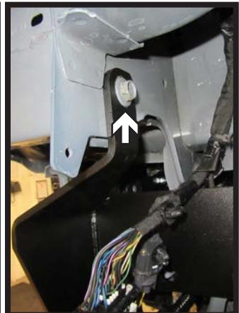
20. Slide the baseplate bracket onto the driver side of the vehicle and reinstall the two (2) M8 bolts with washers (left) and one (1) M10 bolt (right). Leave loose.
