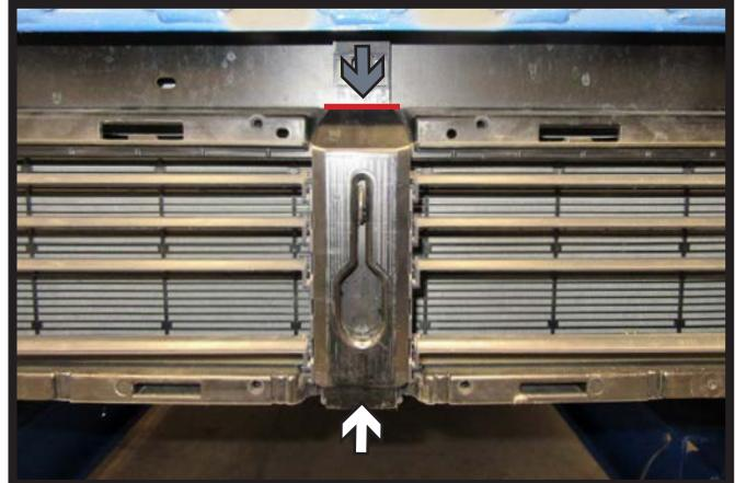
12. **Vehicles without ACC:** Using a reciprocating saw, cut the top of the shutter center piece as shown (gray). Then remove the remaining center piece cover (white).
