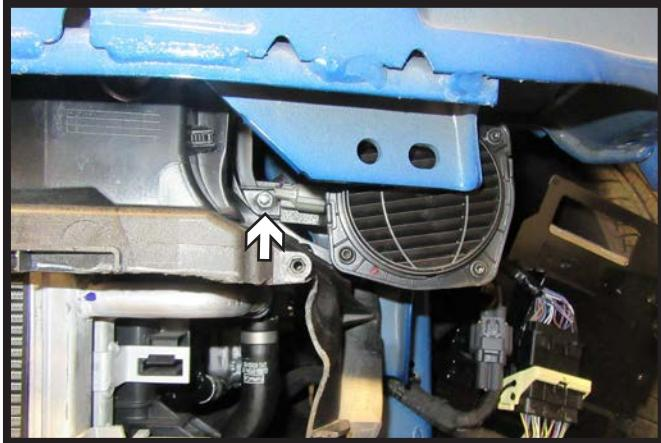
17. Reinstall the pedestrian alert speaker on the driver side of the vehicle. Start the provided 1/4" x 3/4" bolt with nylon nut. Ensure the speaker is as high and towards the center of the vehicle as possible then tighten bolt.
