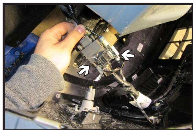
7. As the fascia is removed, unplug the two (2) electrical connections on the passenger side of the vehicle. Set fascia aside to be reinstalled later.
