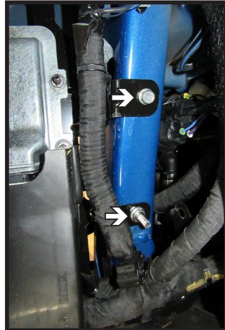
10. Using a 10MM socket, remove the one (1) nut from the top of the black box in front of the wheel on the driver side of the vehicle (left). Then remove the wire loom from the backside bottom bolt. Using a 10MM deep socket, remove the two (2) bolts from the backside (right). Let box hang out of the way for baseplate installation.
