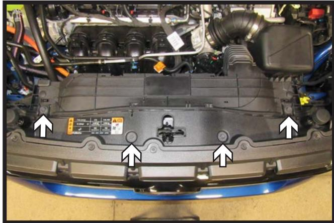
1. Using a 10MM socket, remove the four (4) bolts from the top of the fascia.
