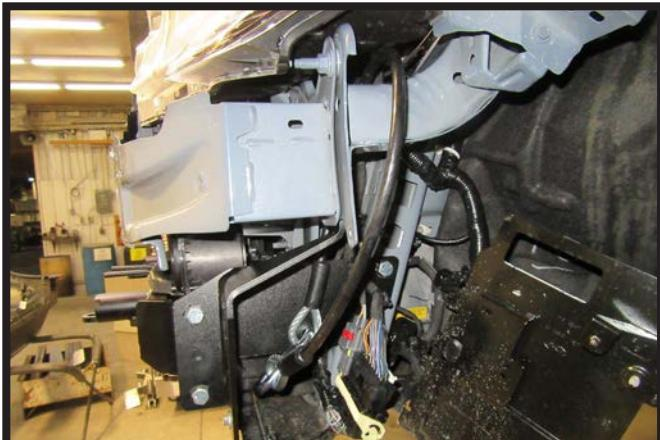
25. Attach the permanent baseplate safety cables to the provided convenience link on the baseplate. The photo above shows the recommended installation of the cables to frame of vehicle. Additional options may interfere with suggested mounting; in this case, secure the cables to a solid piece of the frame as described in the General Information sheet. Be sure the safety cables do not rub against any hoses or moving parts. Do this on **BOTH** sides of the vehicle.
