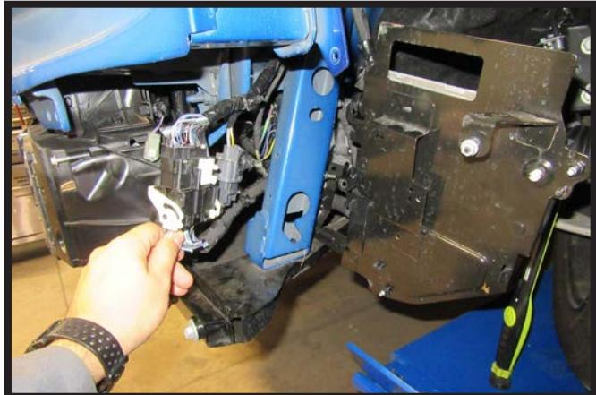
11. Unclip the electrical and wire loom from the front of the black box and the front of the frame on the driver side of the vehicle.
