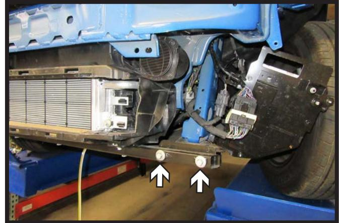
18. Using a 13MM socket, remove the two (2) bolts from the bottom of the frame on the driver side of the vehicle.
