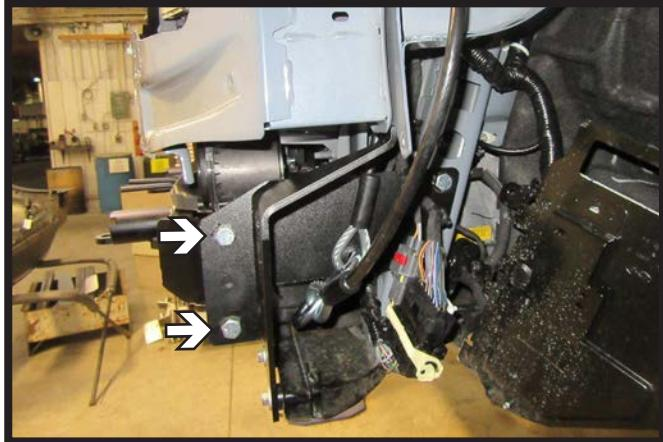
21. Slide the baseplate center piece into place. Install four (4) 1/2" bolts with nylon lock nuts, two (2) on each side. Ensure the center tube is level then tighten all bolts at this time.
