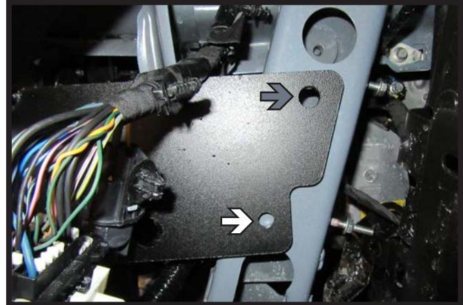
22. Using a 3/8" drill bit, drill out the back bottom hole (white) using the baseplate as a template. If needed use a 1/2" drill bit to ream out the back top hole (gray). Do this on both sides of the vehicle.
