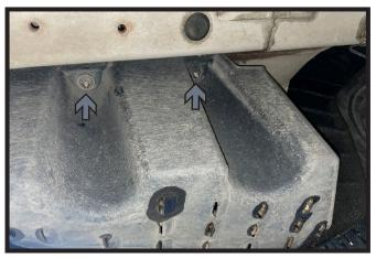
3. Remove the three (3) push pins (white) from the plastic piece on the driver side of the vehicle. Then using a 14MM socket with 10" extension, remove the two (2) nuts (gray). Remove plastic piece and set aside to be reinstalled later.
