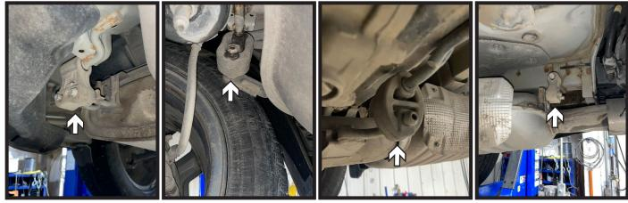
2. Support exhaust using a jack or stand. Remove the four (4) rubber isolators from the exhaust rods on the passenger side of vehicle. Lower exhaust(s) to allow for receiver hitch installation.
