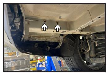
4. Using a wire brush, clean out the side holes on each side of the frame piece. Do this on both sides of the vehicle.
