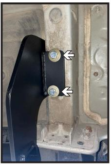
5. Raise the receiver hitch into place and start two (2) 10MM bolts with 7/16" conical washers into the bottom holes. Ensure the teeth of the conical washers are towards the hitch. Leave loose. Do this on both sides of the vehicle.
