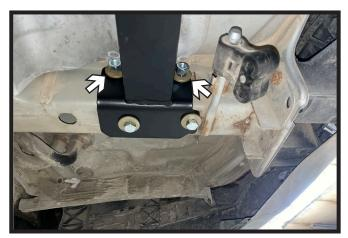
6. Install two (2) 1/2" bolts with 1/2" conical washers and hex nuts into side holes. Ensure the teeth of the conical washers are towards the hitch. Do this on both sides of the vehicle. Tighten all bolts at this time.
