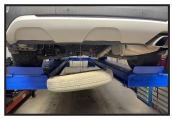
1. Open lift gate of the vehicle. Pull up on the tab to bottom compartment. Lift handle to secondary compartment. Unscrew the cap in the bottom to access the nut holding the spare tire in place. Using the wrench provided with the roadside assistance tools let down the spare tire to allow clearance for receiver hitch installation.
