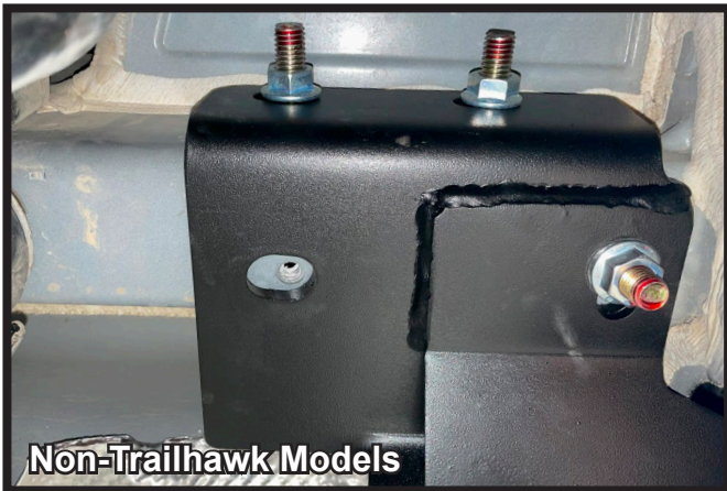
19. Tighten side bolts, alternating between the driver side and passenger side. Once side bolts are tightened, tighten bottom rear bolt on each side of the vehicle.
