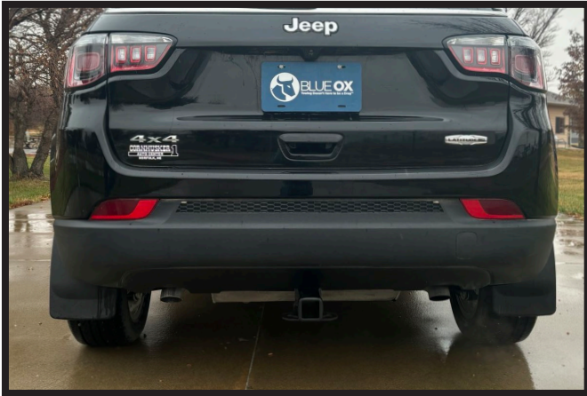
23a. Non-Trailhawk Models Only: Reattach rear fascia to brackets using existing bolts.
