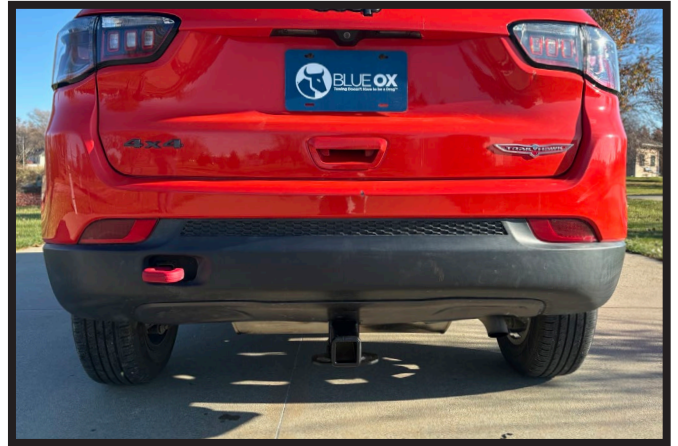
23b. Trailhawk Models Only: Reinstall the rear plastic piece using the provided rivets and reattach rear fascia to brackets using existing bolts.
