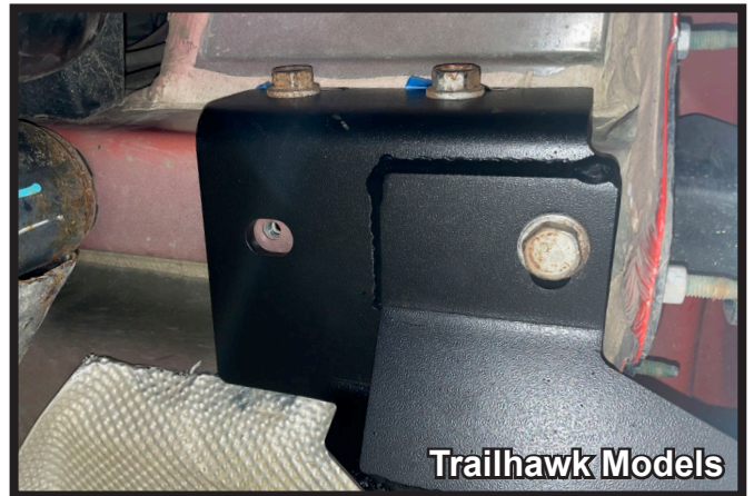
19. Tighten side bolts, alternating between the driver side and passenger side. Once side bolts are tightened, tighten bottom rear bolt on each side of the vehicle.
