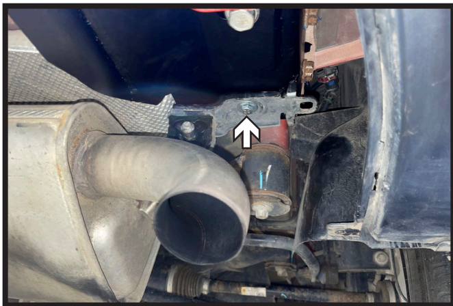
21. Raise the exhaust and reinstall the exhaust bracket on each side of the vehicle using the provided 8MM bolt with conical washer. Ensure the teeth of the conical washer are towards the hitch. Then tighten bottom rear bolts.
