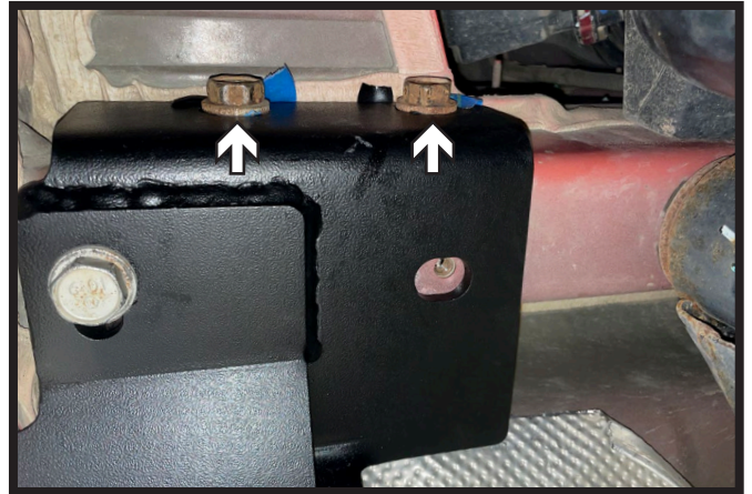
18b. Trailhawk Models Only: Loosely install the existing bolts into the two (2) side holes. Do this on both sides of the vehicle.
