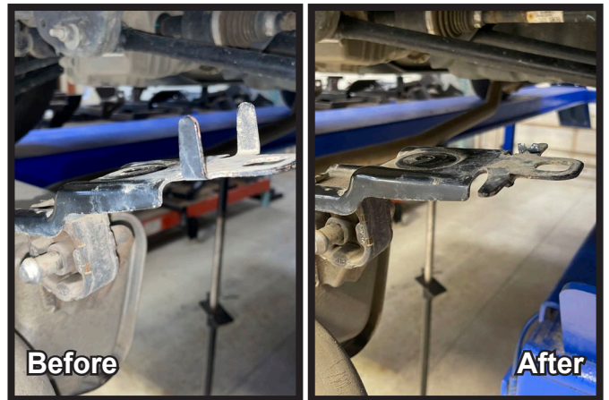
20b. Trailhawk Models Only: Bend down the tabs on the exhaust bracket or use a reciprocating saw to remove the tabs from the exhaust bracket. Do this on both sides of the vehicle.
