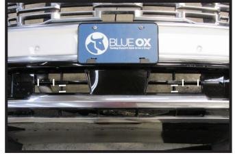
20. Using a reciprocating saw, trim the fascia as indicated on both sides of the vehicle to allow for baseplate clearance.
