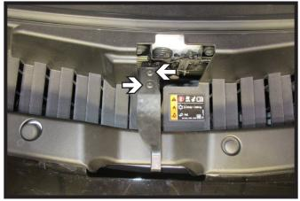
Using a T15 Torx, remove the two (2) screws from the hood latch handle. Remove handle and set aside to be reinstalled later.
