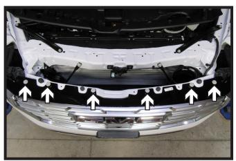
3. Using a 10MM socket, remove the six (6) bolts from the top of the fascia.
