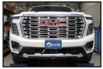
21. Reinstall bumper and air dam. Reattach ACC bracket and wire loom to the bumper. Then reinstall fascia, fascia cover, hood latch handle. Reconnect all electrical connections.
