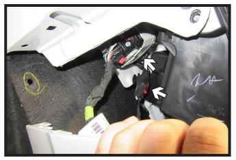
8. Gently pry the fascia loose from the front end of the vehicle. Unplug the two (2) electrical connections on the passenger side behind the facia. Remove the fascia and set aside to be reinstalled later.
