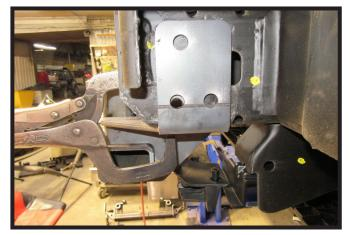
Slide the baseplate onto the vehicle lining up the existing hole on each side as close as possible. Hold in place using large vice grips.
