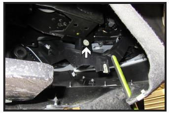
Pull back the bottom of the wheel well liner in front of the tire. Using a 10MM socket, remove the one (1) bolt. Do this on both sides of the vehicle.
