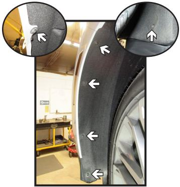
Using a T15 Torx, remove the six (6) screws from the wheel well. There are five (5) along the edge and one (1) in front of the tire. Do this on both sides of the vehicle.
