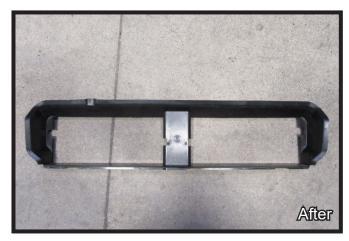
26. Using a reciprocating saw, notch the shutter shroud at each end and in the center as shown to allow for baseplate and electrical rod clearance. Reinstall shroud.
