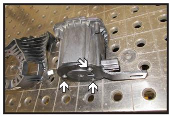
15. Using the existing bolts, attach the provided new mounting bracket to the bottom of the speaker as shown.
