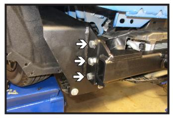
20. Slide the baseplate center piece into place. Install six (6) 1/2" bolts with nylon lock nuts, three (3) on each side. Ensure the center tube is level then tighten all bolts at this time.
