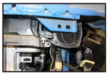
16. Reinstall the pedestrian alert speaker on the driver side of the vehicle. Start the provided 1/4" x 3/4" bolt with nylon nut. Ensure the speaker is as high and towards the center of the vehicle as possible then tighten bolt.
