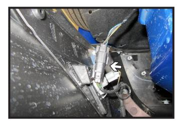
7. As the fascia is removed, unplug electrical connection on the passenger side of the vehicle. Set fascia aside to be reinstalled later.
