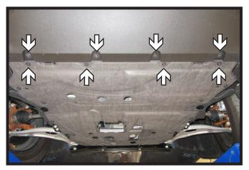
6. Using a T30 Torx, remove the eight (8) bolts from the underside of the fascia.
