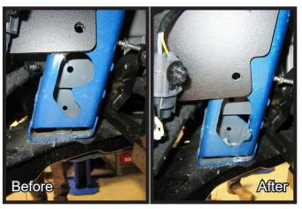
23. Using a pair of large vise grips bend back the frame piece as shown to create an access hole for the nut plate. Do this on both sides of the vehicle.
