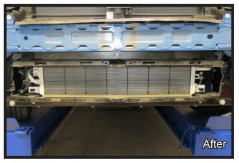
13. Using a reciprocating saw, cut the shutters as indicated to allow for baseplate clearance.
