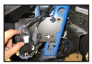
22. Using a 3/8" drill bit, drill out the back bottom hole (white) using the baseplate as a template. If needed use a 1/2" drill bit, ream out the back top hole (gray). Do this on both sides of the vehicle.
