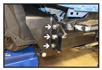
20. Slide the baseplate center piece into place. Install six (6) 1/2" bolts with nylon lock nuts, three (3) on each side. Ensure the center tube is level then tighten all bolts at this time.
