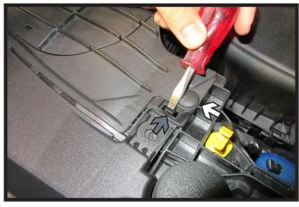
2. Remove the one (1) push pin (white) from the top of the fascia. Then using a flat screw driver, push down on the hook (gray) to release. Do this on both sides of the vehicle.
