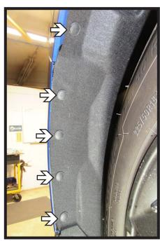
3. Remove the five (5) push pins from the wheel well edge. Do this on both sides of the vehicle.
