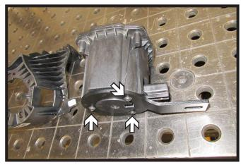
15. Using the existing bolts, attach the provided new mounting bracket to the bottom of the speaker as shown.
