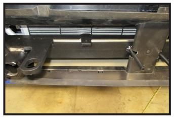
27. **Optional:** Install the breakaway switch to the breakaway bracket on the baseplate using the provided 1/4" bolt and nut.
