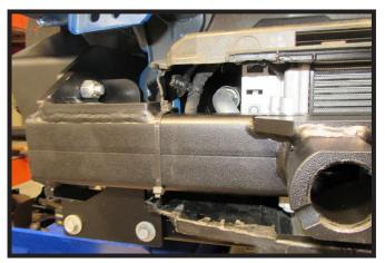
21. Using the provided zip ties, secure the wire loom on the passenger side of the vehicle to the back of the baseplate as shown. Ensure the wire loom is as far away from the radiator tubes as possible.
