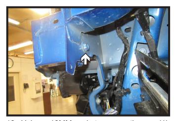
18. Using a 16MM socket, remove the one (1) bolt from behind the bumper on the driver side of the vehicle.
