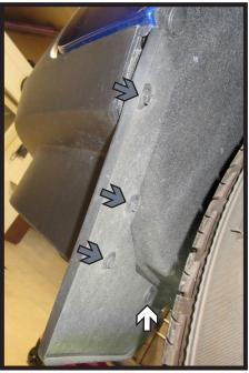
4. Using a 7MM socket, remove the three (3) bolts (gray) and one (1) push pin (white) from the wheel well edge. Do this on both sides of the vehicle.
