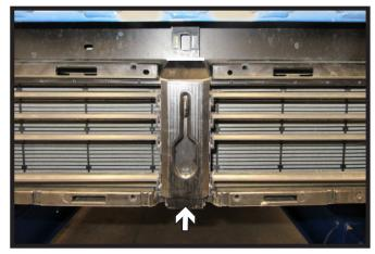
12. Using a reciprocating saw, cut the top of the shutter center piece as shown. Then remove the remaining center piece cover.
