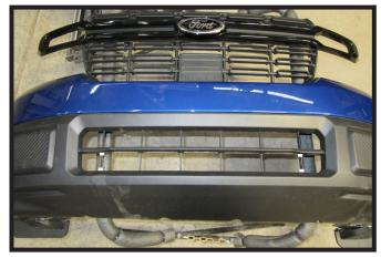
28. Using a reciprocating saw, remove the two (2) vertical slats, one (1) on each side, between the white marks as shown to allow room for the removable tabs and convenience links.
