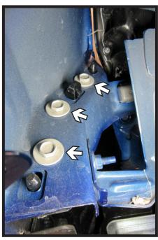
Pull back the wheel well liner. Using a 10MM socket, remove the three (3) bolts from the fascia joint. Do this on both sides of the vehicle.
