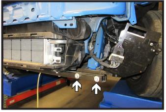
17. Using a 13MM socket, remove the two (2) bolts from the bottom of the frame on the driver side of the vehicle.
