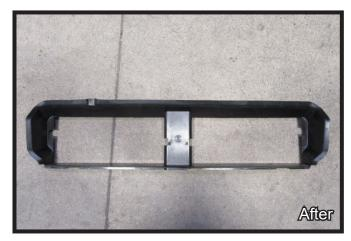
26. Using a reciprocating saw, notch the shutter shroud at each end and in the center as shown to allow for baseplate and electrical rod clearance. Reinstall shroud.
