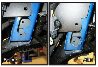
23. Using a pair of large vise grips bend back the frame piece as shown to create an access hole for the nut plate. Do this on both sides of the vehicle.
