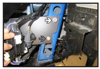
24. Insert nut plate through hole in the frame. Insert a 1/2" bolt into the top hole (white) and a 3/8" bolt into the bottom hole (gray). Bend frame piece back into place. Tighten all bolts. Do this on both sides of the vehicle.
