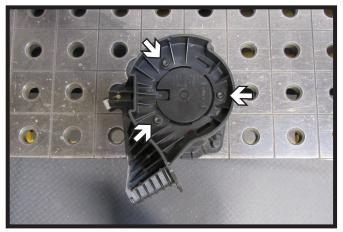
14. Using a T20 Torx, remove the three (3) bolts from the bottom of the pedestrian alert speaker. Remove the mounting bracket from the speaker.
