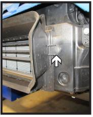
8. Remove the two (2) push pins (white), one (1) on each side of the shroud around the lower shutters. Then using a flat screw driver, release the eight (8) clips around the edge of the shroud (gray). Remove shroud and set aside to be reinstalled later.
