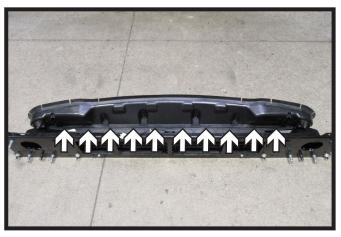
13. Remove the shutter housing from the shutters by unclipping the ten (10) clips on the top, ten (10) on the bottom and one (1) on each side. Remove shutter housing and set aside to be reinstalled later.
