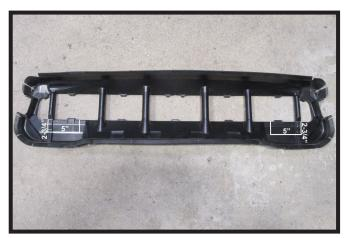
24. Using a reciprocating saw remove the indicated area of the shutter housing to allow clearance for the baseplate and convenience links.
