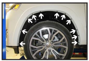
Using an 8MM socket, remove the eleven (11) bolts from the wheel well trim. Do this on both sides of the vehicle.
