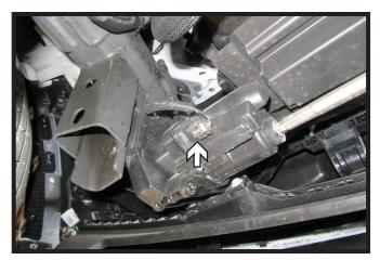
6. Unplug the electrical from the automatic valence on the driver side of the vehicle.
