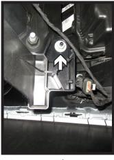
Using a 13MM socket, remove the two
