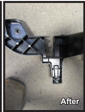
27. Using a reciprocating saw, trim the plastic piece from behind the bumper as shown. Do this on both sides of the piece. Reinstall plastic piece.
