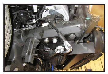
26. Attach the permanent baseplate safety cables to the provided convenience link on the baseplate. The photo above shows the recommended installation of the cables to frame of vehicle. Additional options may interfere with suggested mounting; in this case, secure the cables to a solid piece of the frame as described in the General Information sheet. Be sure the safety cables do not rub against any hoses or moving parts. Do this on BOTH sides of the vehicle.
