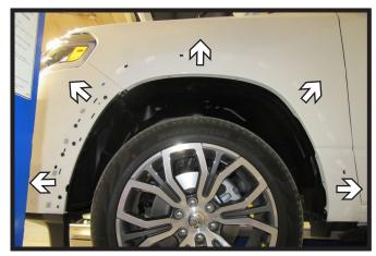
Pull trim outward to release from clips and remove. Set trim aside to be reinstalled later. Remove clips and attach them to trim for easier reinstallation. Do this on both sides of the vehicle.
