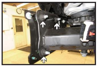
12. Using an 18MM socket, remove the three (3) nuts from the back of the bumper. Do this on both sides of the vehicle. Slide bumper and lower shutter piece off the vehicle and set aside to be reinstalled later.
