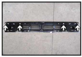
17. Using a 10MM socket, remove the four (4) bolts attaching the shutters to the bumper frame. Remove shutters and set aside to be reinstalled later.
