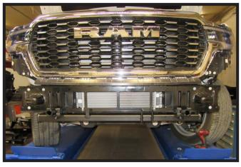
23. Reinstall the bumper piece onto the vehicle.
