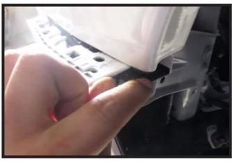
11. Start to remove the fascia at the fascia joint. To release the fascia, push up on the fascia and down on the black piece behind. Do this on both sides of the vehicle. Remove fascia and set aside to be reinstalled later.
