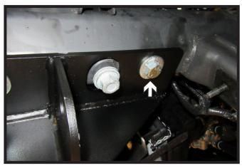
22. Install one (1) 1/2" bolt with flat washer and whiz nut in the back bottom hole of the baseplate. Tighten. Do this on both sides of the vehicle.
