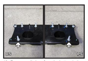
16. Remove coil piece from the bottom bolt on each side. Remove the two (2) bolts from the bumper.
