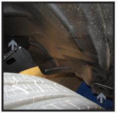
3. Using an 8MM socket, remove the five (5) bolts (white) and four (4) push pins (gray) from the wheel well liner. Remove liner and set aside to be reinstalled later. Do this on both sides of the vehicle.
