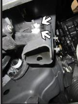
Using a 13MM socket, remover the four (4) nuts, two (2) on each side. Remove valence and set aside to be reinstalled later.
