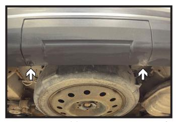
Twist the two (2) screws on the bottom of the rear cover to release. Remove cover and set aside to be reinstalled later.
