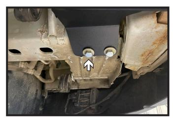
6. Start one (1) 12MM bolt with conical washer into rear hole. Ensure the teeth of the conical washer are towards the hitch. Do this on both sides of the vehicle.
