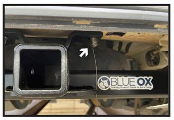
7. **Vehicle without Existing Weldnuts**: Starting on the passenger side of the vehicle feed lead wire from the hole in the rear cross member to the opening at the end of the tube. Place spacer plate onto wire then attach lead wire to the end of the 1/2" carriage bolt (right). Pull bolt and spacer plate through the frame. Ensure spacer plate is sitting flush against inner frame and the bolt is hanging vertically (left). Repeat on the driver side of the vehicle.
