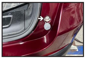
Using a 10MM socket, remove the one (1) bolt at the bottom of the rear fascia. Do this on both sides of the vehicle. Remove the rear fascia and set aside to be reinstalled later.
