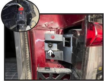
9. Using a T30 Torx, remove the bolt next to the tail light. As the tail light is removed, unplug electrical connection (inset) on the back of the light. Set tail light aside to be reinstalled later. Do this on both sides of the vehicle.
