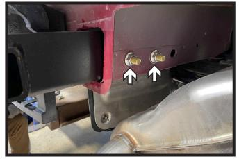
Clean out any road debris from inside of the frame on both sides of the vehicle. Slide the receiver hitch into the frame. Start two (2) 1/2" carriage bolts with flat washers and lock nuts in the side frame holes. Do this on both sides of the vehicle. L Models: Use the set of holes farthest from the hitch cross bar. Non-L Models: Use the set of holes
