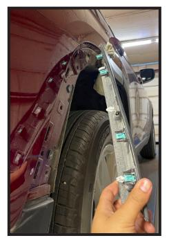
3. Pull back the wheel well trim, releasing the push pins, past the fascia joint. Prop trim away from the vehicle using a soft cloth. Do this on both sides of the vehicle.
