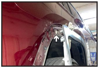
4. Using a 10MM socket, remove the one (1) bolt from the fascia joint. Do this on both sides of the vehicle.
