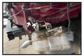
Using a 13MM socket, remove the two
