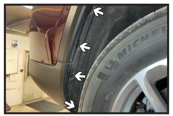
Using an 8MM socket, remove the four (4) bolts from along the edge of the rear wheel well. Do this on both sides of the vehicle.
