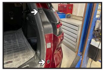
6. Lift tailgate. Using a flat screw driver, remove the two (2) plastic covers next to the tail light. Do this on both sides of the vehicle.
