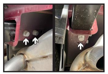
Using a 21MM socket, remove the three
