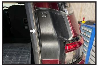
7. Using a flat screw driver, remove the plastic piece next to the tail light. Set aside to be reinstalled later. Do this on both sides of the vehicle.
