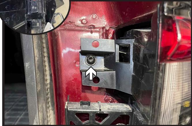
9. Using a T30 Torx, remove the bolt next to the tail light. As the tail light is removed, unplug electrical connection (inset) on the back of the light. Set tail light aside to be reinstalled later. Do this on both sides of the vehicle.
