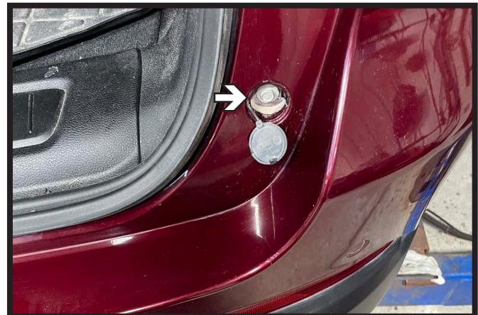
8. Using a 10MM socket, remove the one (1) bolt at the bottom of the rear fascia. Do this on both sides of the vehicle. Remove the rear fascia and set aside to be reinstalled later.
