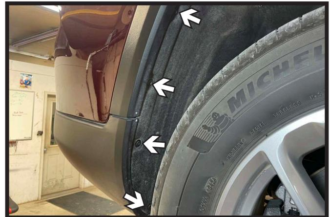
2. Using an 8MM socket, remove the four (4) bolts from along the edge of the rear wheel well. Do this on both sides of the vehicle.
