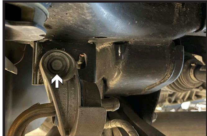
11. Using a 13MM socket, remove the one (1) bolt from the exhaust bracket near the rear tire on the passenger side of the vehicle. Lower exhaust.
