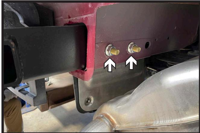
13. Clean out any road debris from inside of the frame on both sides of the vehicle. Slide the receiver hitch into the frame. Start two (2) 1/2" carriage bolts with flat washers and lock nuts in the side frame holes. Do this on both sides of the vehicle. **L Models:** Use the set of holes farthest from the hitch cross bar. **Non-L Models:** Use the set of holes nearest to the hitch cross bar.
