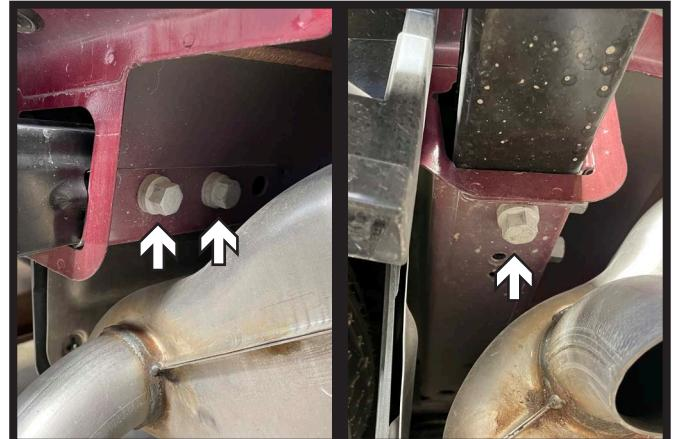
12. Using a 21MM socket, remove the three (3) bolts from the rear bumper. There are two (2) on the side and one (1) on the bottom. Do this on both sides of the vehicle. Remove rear bumper, it will not be reinstalled.
