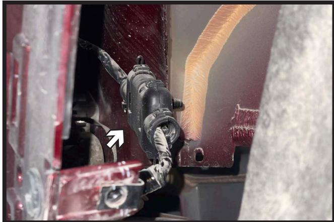
5. Unclip the electrical connection from behind the rear tire. Do this on both sides of the vehicle.
