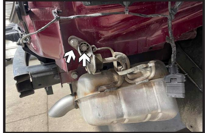
10. Using a 13MM socket, remove the two (2) bolts from the exhaust bracket on the passenger side of the vehicle.
