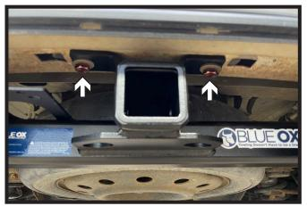
8b. Vehicle with Existing Weldnuts: Insert two (2) 12MM bolts into the rear holes. Ensure the teeth of the conical washer are towards the hitch. Then tighten all bolts.
