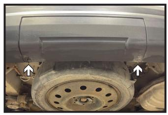
Twist the two (2) screws on the bottom of the rear cover to release. Remove cover and set aside to be reinstalled later.
