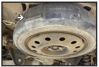
Loosen spare tire and rotate the cover slightly so the protruding piece is out of the way of the receiver hitch. Re-secure spare tire.
