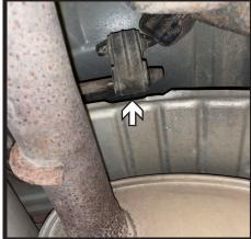
2. Support exhaust using a jack or stand. Remove the three (3) rubber isolators from the exhaust rods on the passenger side of vehicle. There is one (1) on each side of the exhaust and one (1) towards the front. If vehicle is equipped with dual exhaust, repeat step on the driver side of the vehicle. Lower exhaust(s) to allow for receiver hitch installation.
