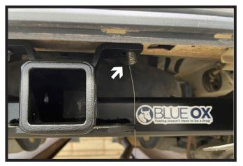
7. **Vehicle without Existing Weldnuts**: Starting on the passenger side of the vehicle feed lead wire from the hole in the rear cross member to the opening at the end of the tube. Place spacer plate onto wire then attach lead wire to the end of the 1/2" carriage bolt (right). Pull bolt and spacer plate through the frame. Ensure spacer plate is sitting flush against inner frame and the bolt is hanging vertically (left). Repeat on the driver side of the vehicle.
