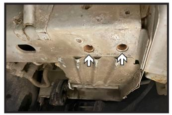
Clean out existing bolt holes. Then run a M12 x 1.75 tap through the holes. Verify that the provided 12MM bolts will fit in the holes after they have been cleaned. Do this on both sides of the vehicle.
