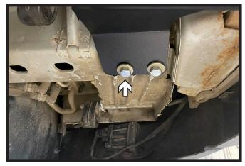
6. Start one (1) 12MM bolt with conical washer into rear hole. Ensure the teeth of the conical washer are towards the hitch. Do this on both sides of the vehicle.
