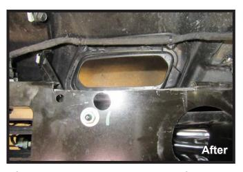
14. Using a reciprocating saw trim the indicated area from the metal piece on the back of the bumper as shown. Do this on both sides of the vehicle.
