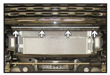
15. Remove the four (4) push pins from rubber piece below grille and remove. It will not be reinstalled. Then using a reciprocating saw, cut a straight line across the plastic piece to remove the indicated area.
