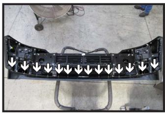
4. Using a 10MM socket, remove the fourteen (14) nuts from the bottom of the bumper. Remove bumper valence and set aside to be reinstalled later.
