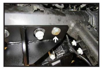
19. Install the 1/2" x 1-1/2" bolt with flat washer and whiz nut into the bottom back hole. Fully tighten all bolts at this time starting with the side bolt, then back bottom bolt, and finally the front bottom bolt. Do this on both sides of the vehicle.
