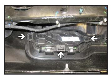
Vehicles without Tow Hooks: Unclip the three (3) clips from the tow hook cover and push towards the back of the bumper to remove. Do this on both sides of the bumper.
