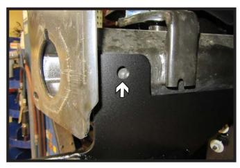
17. Using a 1/2" drill bit, drill the bottom hole and side hole using the baseplate as a template. Do this on both sides of the vehicle.
