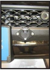
20. Reinstall the automatic valence and bumper. Using a 1-1/2" hole saw drill a hole in the bumper on the driver side for the electrical plug as shown. Hold plug in place, using a 1/4" drill bit, drill the two (2) holes in the bumper for the bolts using the plug as a template. Install plug using provided hardware.
