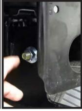
18. Place spacer plate onto 1/2" carriage bolt. Insert bolt and plate through access hole in the front of the vehicle frame. Install bolt and plate into side hole in baseplate and attach 1/2" flange whiz nut. Hand tighten. Do this on both sides of the vehicle.
