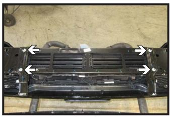
Using a 13MM socket, remove the four (4) nuts from the brackets on the back of the bumper. Remove brackets, they will not be reinstalled.
