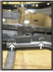
5. Remove the four (4) push pins, two (2) on each side, from the rubber piece on the top of the bumper.
