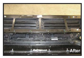
11. Unclip the wire loom from the bottom of the bracket on the back side of the bumper and reinstall to the forward side of the bracket as shown.
