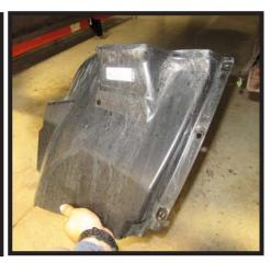
1. Using an 8MM socket, remove the five (5) bolts from the wheel well. Remove plastic piece and set aside to be reinstalled later. Do this on both sides of the vehicle.
