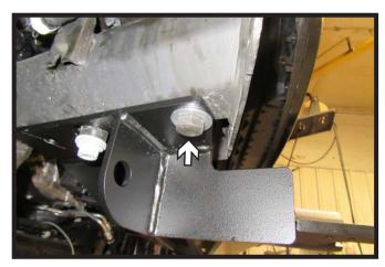
16. Raise baseplate into place and start the 14MM bolt with flat washer and nylon lock nut, hand tighten. Do this on both sides of the vehicle.
