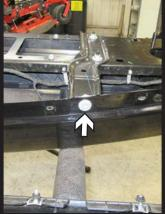
6. Pull back rubber piece. Using a T40 Torx, remove the three (3) bolts from the bumper. There are two (2) on the top and one (1) on the bottom. Do this on both sides of the bumper.
