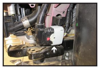
19. Unclip electrical loom from the frame on driver side of the vehicle to allow for installation of support plate.
