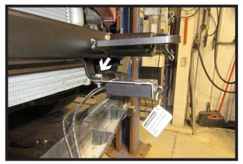
25. **Optional Breakaway**: Attach breakaway switch to the driver side of the baseplate as shown using the provide hardware.
