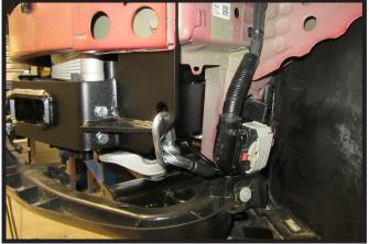
21. Reattach electrical loom to frame on the driver side of the vehicle.
