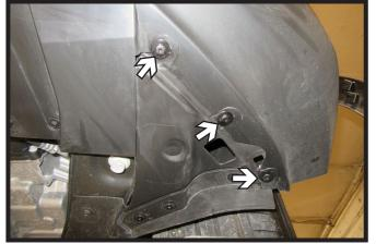
5. Using a T15 Torx, remove the three (3) bolts from the bottom of the fascia in front of the tire. Do this on both sides of the vehicle.
