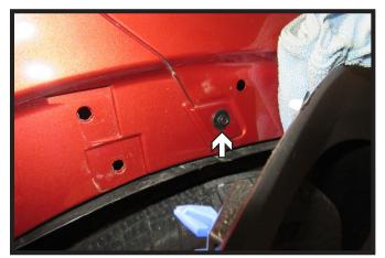
3. Using a 7MM socket, remove the one (1) bolt from the fascia joint. Do this on both sides of the vehicle.
