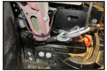
22. Attach the permanent baseplate safety cables to the provided convenience link on the baseplate. The photo above shows the recommended installation of the cables to frame of vehicle. Additional options may interfere with suggested mounting; in this case, secure the cables to a solid piece of the frame as described in the General Information sheet. Be sure the safety cables do not rub against any hoses or moving parts. Do this on **BOTH** sides of the vehicle.
