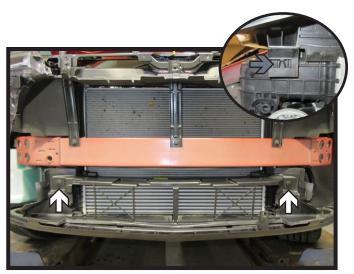
Remove the two (2) push pins, one (1) on each side from the plastic shroud. Then release the clip from the bottom of shroud, there is one (1) on each side (inset). Remove shroud, it will not be reinstalled.
