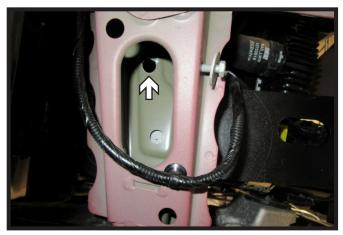
18. Using a 1/4" drill bit, create starter hole in frame on the passenger side of the vehicle. Then using a 1/2" drill bit, drill out top hole in frame.
