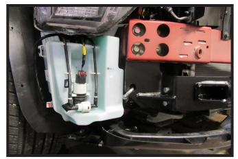
23. Reinstall windshield washer fluid reservoir, reconnecting all lines and electrical connections.
