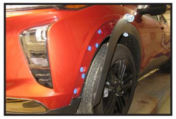
Pull back the wheel well trim, releasing the nine (9) push pins, past the fascia joint. Prop trim away from the vehicle using a soft cloth. Do this on both sides of the vehicle.
