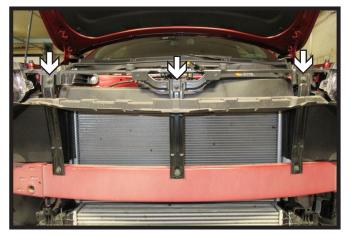
Optional: Reattach bumper to support brackets, leave loose. Then using a 10MM socket, loosen the top three (3) support bracket bolts.
