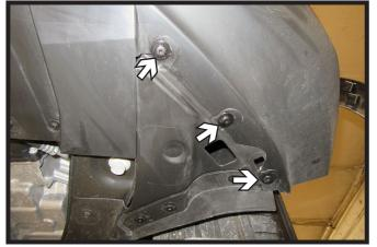
5. Using a T15 Torx, remove the three (3) bolts from the bottom of the fascia in front of the tire. Do this on both sides of the vehicle.
