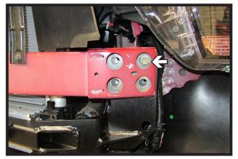
14. Slide the baseplate onto the vehicle between the frame and the bumper. Start one (1) existing 10MM bolt in the top outer hole. Do this on both sides of the vehicle. Ensure the holes on the bumper line up with the baseplate. If the six (6) support bracket bolts were loosened, tighten at this time.
