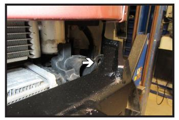
16. **Optional**: If needed trim the indicated corner plastic piece to allow for baseplate clearance.
