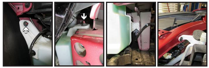
9. Using a 10MM socket, remove the two (2) nuts (white), one (1) bolt (gray), and one (1) push pin (black) from the windshield washer fluid reservoir on the passenger side of the vehicle. Disconnect and plug all lines. Disconnect the two (2) electrical connections. Remove reservoir and set aside to be reinstalled later.
