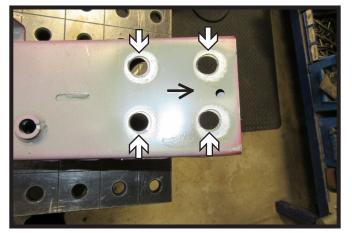
12. **Optional**: If needed slightly slot the four (4) holes in the bumper towards the outside. Do this on both sides of the bumper.
