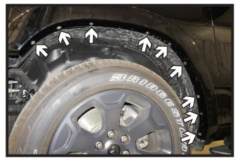
Using an 8MM socket, remove the nine
