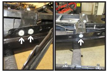
Pull back rubber piece. Using a T40 Torx, remove the three (3) bolts from the bumper. There are two (2) on the top and one (1) on the bottom. Do this on both sides of the bumper.
