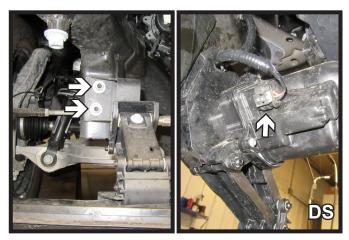
10. Using a 13MM socket, remove the two (2) nuts from the automatic valence. Do this on both sides of the vehicle. Unplug the electrical connection on the driver side and remove valence and set aside to be reinstalled later.
