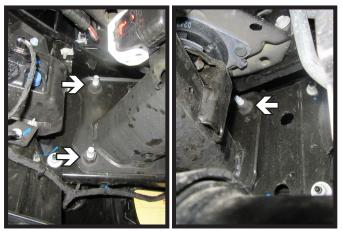
Using an 18MM socket, remove the three (3) bolts from the back of the bumper. Do this on both sides of the vehicle. Remove bumper and set aside to be reinstalled later.
