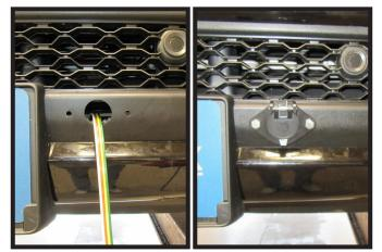
Reinstall the automatic valence and bumper. Using a 1-1/4" hole saw drill a hole in the bumper on the driver side for the electrical plug as shown. Hold plug in place, using a 1/4" drill bit, drill the two (2) holes in the bumper for the bolts using the plug as a template. Install plug using provided hardware.
