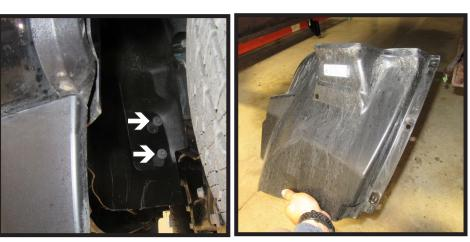
1. Using an 8MM socket, remove the five (5) bolts from the wheel well. Remove plastic piece and set aside to be reinstalled later. Do this on both sides of the vehicle.
