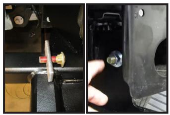
17. Place spacer plate onto 1/2" carriage bolt. Insert bolt and plate through access hole in the front of the vehicle frame. Install bolt and plate into side hole in baseplate and attach 1/2" flange whiz nut. Hand tighten. Do this on both sides of the vehicle.
