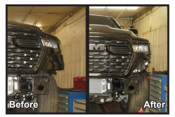
14. Starting in the wheel well, pull outward to release the three (3) clips attaching the fascia panel below the headlight. Do this on both sides of the vehicle.
