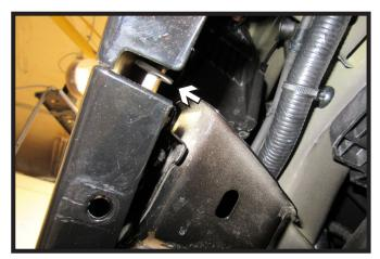
13. Using a 10MM socket, remove the one (1) bolt from the fascia joint. Do this on both sides of the vehicle.
