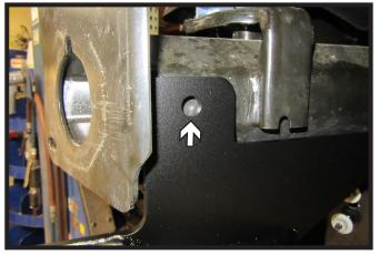
16. Using a 1/2" drill bit, drill the bottom hole and side hole using the baseplate as a template. Do this on both sides of the vehicle.
