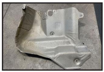
Using a reciprocating saw trim the heat shield as indicated to allow for receiver hitch clearance. Repeat this processes with heat shield on other side of the vehicle.
