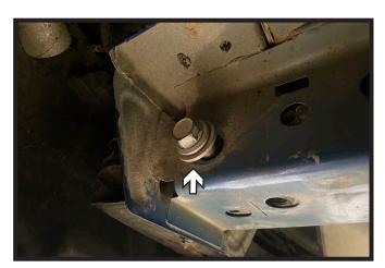
7. Using a 21MM socket, remove the one (1) bolt from the side of the frame. Do this on both sides of the vehicle.
