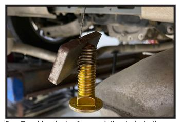
9. Feed lead wire from existing hole in the bottom of the frame to the hole at the rear of the frame. Place spacer plates onto wire then attach lead wire to the end of the 1/2" carriage bolt (inset). Pull bolt and spacer plate through the frame. Repeat process with hole in the side of the frame. Ensure spacer plates are sitting flush against inner frame. Do this on both sides of the vehicle.
