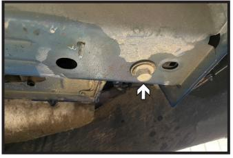
6. Using a 21MM socket, remove the one (1) bolt from the bottom of the frame. Do this on both sides of the vehicle.
