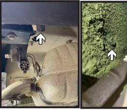
4. Using a 7MM socket, remove the two (2) bolts, one (1) along and one (1) inside the wheel well. Remove heat shield and set aside to be reinstalled later. Do this on both sides of the vehicle.
