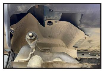
8. Raise heat shield back into place. Do this on both sides of the vehicle.
