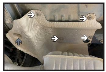
3. Using a 10MM socket, remove the four (4) nuts (white) and one (1) bolt (gray) from the heat shield. Do this on both sides of the vehicle.
