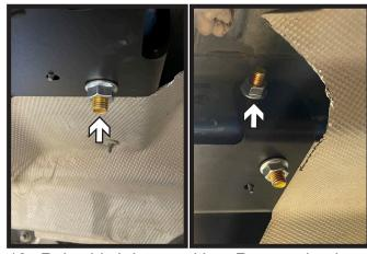
Raise hitch into position. Remove lead wires and loosely install a 1/2" whiz flange nut onto each bolt. Do this on both sides of the vehicle.
