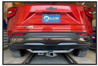
3. Raise hitch into position. Remove lead wires and loosely install 1/2" whiz flange nut onto each bolt. Then tighten all bolts.
