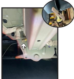
2. Place spacer plate onto wire then attach lead wire to the end of the 1/2" carriage bolt (inset). Pull bolt and spacer plate through the frame. Repeat process with second bolt hole. Do this on both sides of the vehicle. Ensure spacer plates are sitting flush against inner frame and the bolts are hanging vertically. Do this on both sides of the vehicle.
