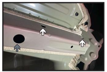
Starting with the rear hole, feed lead wires from holes in the side of the frame (white) to the large access hole (gray) or rear frame hole if available. Do this on both sides of the vehicle.
