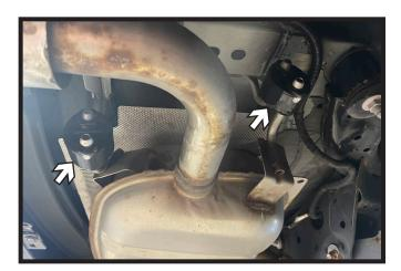
Support exhaust using a jack or stand. Remove the four (4) rubber isolators, two (2) on each side, from exhaust rods. Lower exhaust to allow receiver hitch installation.
