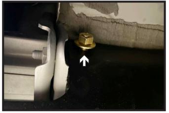
7. **Option 1**: For vehicles with a weld nut in the frame, install one (1) 12MM bolt with conical washer into the rear hole on each side of the vehicle.
