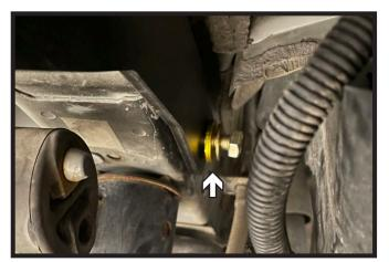
Raise hitch into position. Install one (1)
