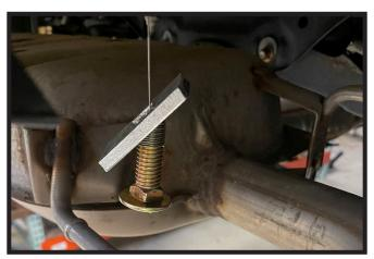
5. **Vehicle without Weld Nut**: If the vehicle does not have a weld nut in the rear frame hole then feed the lead wire from rear frame hole to the forward access hole. Place spacer plates onto wire then attach lead wire to the end of the 1/2" carriage bolt. Pull bolt and spacer plate through the frame. Repeat process with second bolt hole. Ensure spacer plates are sitting flush against inner frame and the bolts are horizontal. Do this on both sides of the vehicle.
