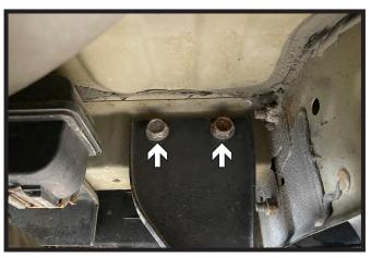
3. Using an 18MM socket, remove the four (4) bolts from the tow hook/bracket on the passenger side of the vehicle. Remove bracket, it will not be reinstalled.
