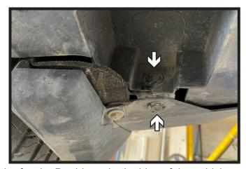
1. Remove the four (4) push pins from bottom of the fascia. Do this on both sides of the vehicle.
