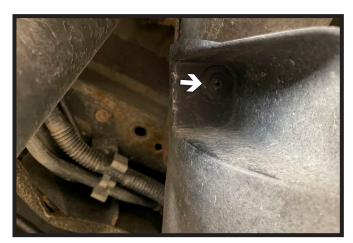
2. Using a Phillips screwdriver, remove the one (1) screw from the rear panel on the under side of the fascia. Remove panel, it will not be reinstalled. Do this on both sides of the vehicle.
