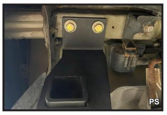
6. Raise hitch into place. Install the five (5) M12-1.25 bolts with conical washer into the existing holes. There are two (2) on the passenger side and three (3) on the driver side. Tighten all bolts.
