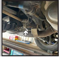
4. Support exhaust using a jack or stand. Remove the three (3) rubber isolators from the exhaust rods, one (1) on each side or the vehicle and one (1) in the center. Lower exhaust to allow receiver hitch installation.
