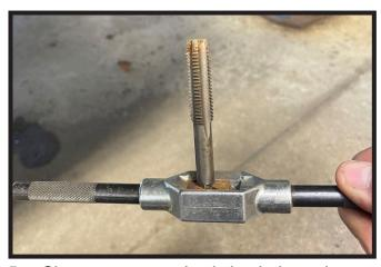
5. Clean area around existing holes using a wire brush. Then run a 12MM x 1.25 tap through the existing holes. Do this on both sides of the vehicle.
