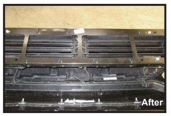
11. Unclip the wire loom from the bottom of the bracket on the back side of the bumper and reinstall to the forward side of the bracket as shown.
