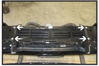
7. Using a 13MM socket, remove the four (4) nuts from the brackets on the back of the bumper. Remove brackets, they will not be reinstalled.
