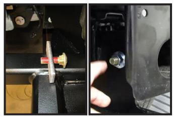
18. Place spacer plate onto 1/2" carriage bolt. Insert bolt and plate through access hole in the front of the vehicle frame. Install bolt and plate into side hole in baseplate and attach 1/2" flange whiz nut. Hand tighten. Do this on both sides of the vehicle.
