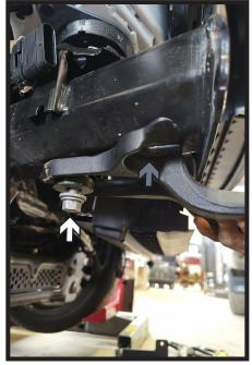
12. **Trucks with Tow Hooks:** Using an 18MM socket remove the front bolt (gray), and then using a 21MM socket remove the back bolt (white) attaching the tow hook to the frame. Do this on both sides of the vehicle. The tow hooks will not be reinstalled.
