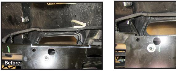
14. Using a reciprocating saw trim the indicated area from the metal piece on the back of the bumper as shown. Do this on both sides of the vehicle.
