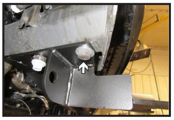
15. Raise baseplate into place and start the 14MM bolt with flat washer and nylon lock nut, hand tighten. Do this on both sides of the vehicle.
