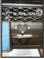
19. Reinstall the automatic valence and bumper. Using a 1-1/2" hole saw drill a hole in the bumper on the driver side for the electrical plug as shown. Hold plug in place, using a 1/4" drill bit, drill the two (2) holes in the bumper for the bolts using the plug as a template. Install plug using provided hardware.
