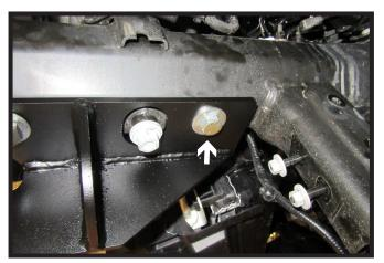
18. Install the 1/2" x 1-1/2" bolt with flat washer and whiz nut into the bottom back hole. Fully tighten all bolts at this time starting with the side bolt, then back bottom bolt, and finally the front bottom bolt. Do this on both sides of the vehicle.
