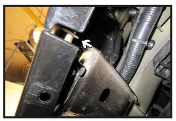
13. Using a 10MM socket, remove the one (1) bolt from the fascia joint. Do this on both sides of the vehicle.
