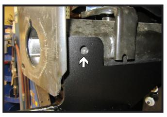
16. Using a 1/2" drill bit, drill the bottom hole and side hole using the baseplate as a template. Do this on both sides of the vehicle.
