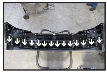
Using a 10MM socket, remove the fourteen (14) nuts from the bottom of the bumper. Remove bumper valence and set aside to be reinstalled later.
