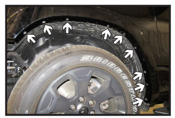
12. Using an 8MM socket, remove the nine (9) bolts from the fender trim. Do this on both sides of the vehicle. Pull up and out on the fender trim to release the clips on the back side. Remove fender trim and set aside to be reinstalled later.
