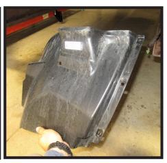
1. Using an 8MM socket, remove the five (5) bolts from the wheel well. Remove plastic piece and set aside to be reinstalled later. Do this on both sides of the vehicle.
