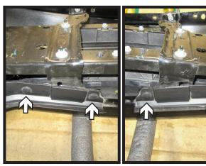
5. Remove the four (4) push pins, two (2) on each side, from the rubber piece on the top of the bumper.
