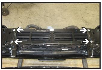
Using a 13MM socket, remove the four (4) nuts from the brackets on the back of the bumper. Remove brackets, they will not be reinstalled.
