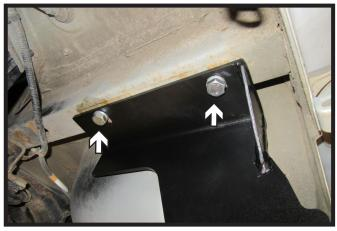
Raise the receiver hitch into place so the holes on the hitch line up with the existing holes in the frame. Install the two (2) 12MM bolts with conical washers. Do this on both sides of the vehicle.
