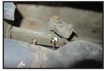
Remove rubber isolator from exhaust rod on passenger side of the vehicle. Lower exhaust.
