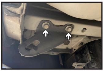
Using a 17MM socket with 8" extension, remove the two (2) bolts from the tie down bracket on the driver side of the vehicle. Remove bracket and set aside to be given to the customer. The bracket will not be reinstalled.
