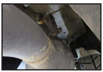
Raise the exhaust back into place and reinstall the rubber isolator.
