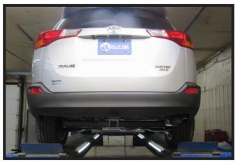
If present, hold rear panel up and trim and to allow clearance for receiver hitch and reinstall or return to customer.
