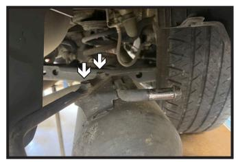
Using a 12MM socket, remove the two
