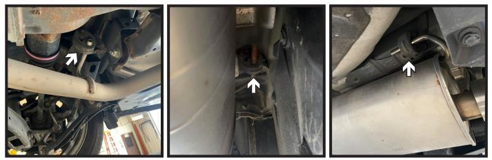
1. Support the exhaust and remove the three (3) rubber isolators from exhaust rods. Lower exhaust to allow receiver hitch installation.
