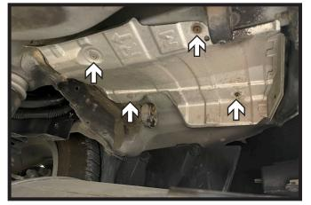
Using a 10MM socket, remove the four (4) bolts from the heat shield on the passenger side of the vehicle. Remove shield and set aside as it can be reinstalled later.
