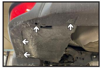
4. Remove the four (4) push pins from the underside of the vehicle on the driver side.
