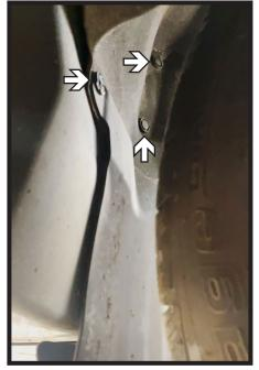
5. Remove the three (3) push pins from behind the tire on the driver side of the vehicle.
