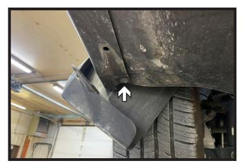
6. Rotate mud flap outward and remove the one (1) push pin from behind the wheel on the driver side of the vehicle. Remove plastic cover on driver side and set aside to be reinstalled later.
