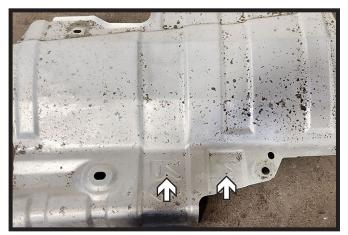
10. **Optional**: Using a 5/8" drill bit, drill out the two (2) dimples in the heat shield and reinstall on the passenger side of the vehicle using existing hardware.
