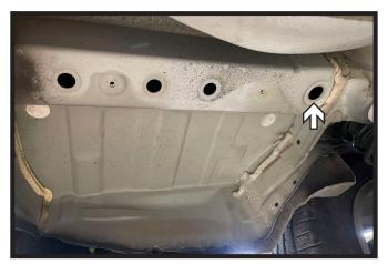
8. Using a 1-1/4" hole saw, drill out the forward most hole to create an access hole. Do this on both sides of the vehicle.
