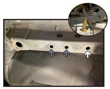
9. Starting with the rear hole, run a lead wire from the rear hole (white) to the access hole. Place a spacer plate onto the wire then attach the lead wire to the end of the 1/2" carriage bolt (inset). Pull bolt through the frame. Ensure the spacer plate is sitting flush against inner frame and the bolt is hanging vertically. Do this for the remaining two (2) holes (gray). Do this on both sides of the vehicle.
