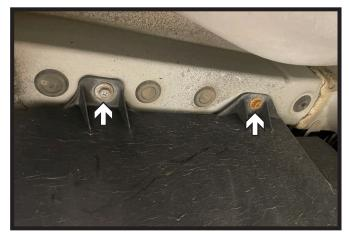
3. Using a 10MM socket, remove the two (2) bolts from the plastic cover on the driver side of the vehicle.
