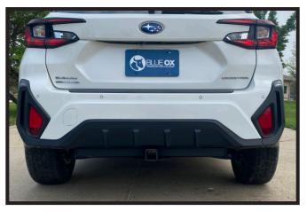
7. Raise hitch into position. Remove lead wires and loosely install 1/2" whiz flange nut onto each bolt. Do this on both sides of the vehicle. Then tighten all bolts.
