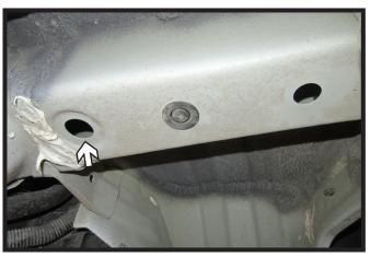
2. Using a die grinder enlarge forward holes so there is enough room for the 1" x 3" x 1/4" spacer plate with 1/2" square hole. Do this on both sides of the vehicle.
