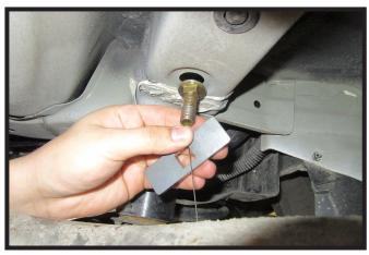
Place spacer plate on bolt and attach lead wire. Feed bolt, then spacer plate through forward hole. Do this on both sides of the vehicle.
