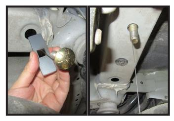
4. Pull bolt and spacer plate through forward hole to rear hole. Do this on both sides of the vehicle.
