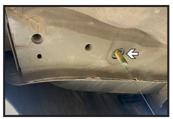
6. Attach lead wire to 7/16" carriage bolt and feed through hole in spacer plate. Insert bolt, then long end of spacer plate through hole in the frame. Ensure spacer plate is sitting flush against inner frame and the bolt is hanging vertically. Do this on both sides of the vehicle.
