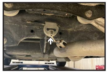
4. Support exhaust using a jack or stand. Remove the two (2) rubber isolators from the exhaust rods, one (1) on the passenger side and one (1) in the center of the vehicle. Lower exhaust to allow receiver hitch installation.
