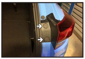
Remove the two (2) plastic caps next to the tail light. Do this on both sides of the vehicle.
