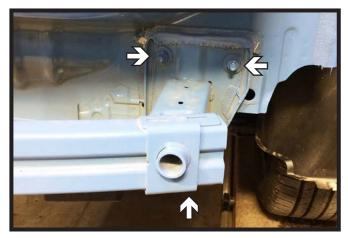
Using a 15MM socket, remove the three
