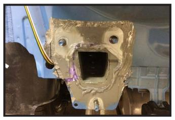
18. Apply clear 100% silicone around the frame hole as shown. Do this on both sides of the vehicle.
