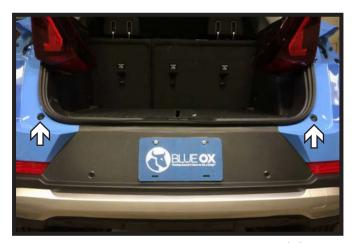
4. Using a T15 Torx, remove the two (2) bolts from below the trail light housing. There is one (1) on each side of the vehicle.
