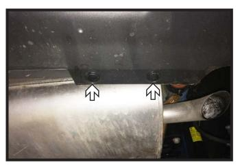
10. Remove the two (2) push pins from the underside of the vehicle. Do this on both sides of the vehicle.
