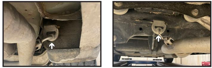
4. Support exhaust using a jack or stand. Remove the two (2) rubber isolators from the exhaust rods, one (1) on the passenger side and one (1) in the center of the vehicle. Lower exhaust to allow receiver hitch installation.
