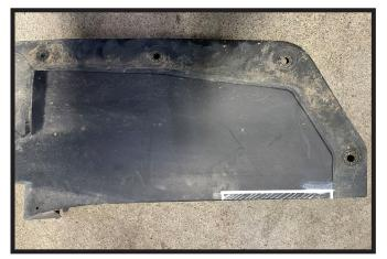
11. Using a reciprocating saw trim the plastic piece from the driver side of the vehicle as shown.
