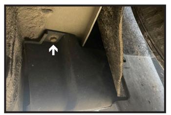
3. Using a 10MM socket, remove the one (1) bolt next to the wheel well on the driver side of the vehicle. Remove plastic piece and set aside to be reinstalled later.
