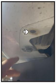
7. Remove the one (1) push pin from the passenger side of the vehicle. Rotate plastic piece to allow for installation of remaining bolts.
