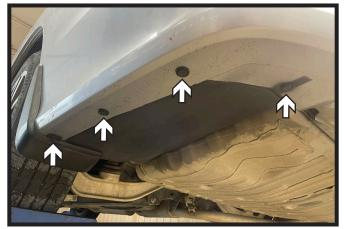
1. Remove the four (4) push pins from the underside of the rear fascia on the driver side of the vehicle.
