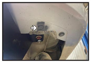
10. Rotate plastic piece on passenger side of the vehicle back into place and reinstall push pin.
