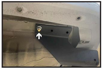
Feed lead wires through rear hole in receiver hitch on both sides. Raise hitch into place. Remove lead wires and loosely install 7/16" whiz flange nut onto each bolt. Leave loose.
