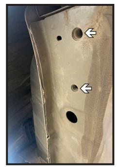
5. Using WD40 or similar product, clean bolt holes and treads for receiver hitch installation. Do this on both sides of the vehicle.
