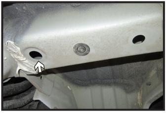
2. Using a die grinder enlarge forward holes so there is enough room for the 1" x 3" x 1/4" spacer plate with 1/2" square hole. Do this on both sides of the vehicle.
