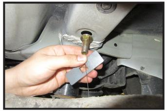
5. Place spacer plate on bolt and attach lead wire. Feed bolt, then spacer plate through forward hole. Do this on both sides of the vehicle.
