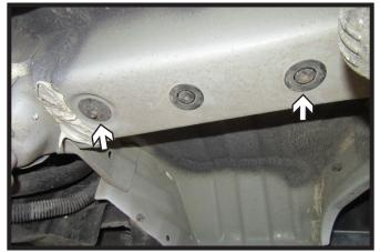
1. Remove the two (2) rubber plugs from the frame rail. Do this on both sides of the vehicle.
