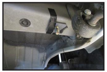
Do not remove lead wire. Hold receiver hitch up to frame. Determine if the 1-1/2" x 2" x 1/4" is needed to level hitch. If needed, tape spacer plate to frame as shown. Do this on both sides of the vehicle.
