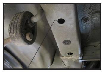
3. Feed wire through frame from rear hole to forward hole. Slide spacer plate onto 1/2" bolt and attach lead wire to end of bolt. Do this on both sides of the vehicle.
