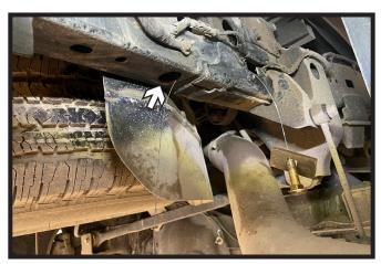
1. Feed lead wire from hole in bottom of the frame to the access hole on the outside of the frame as shown. Place 1-1/2" x 3" spacer plate onto 5/8" carriage bolt. Attach lead wire to the end of the bolt. Do this on both sides of the vehicle.
