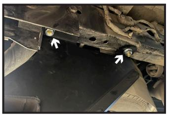
6. Raise receiver hitch into place. Remove lead wire from rear bolt and carefully secure a 5/8" lock nut to each bolt. Do not fully tighten. Do this on both sides of the vehicle.
