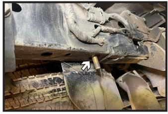
Pull bolt through the frame. Ensure the spacer plate is sitting flush against inner frame and the bolt is hanging vertically. Do this on both sides of the vehicle.
