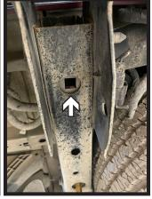
3. Slide the 2-1/8" x 2-1/8" spacer plate through the end of the frame and line up the plate with the hole in the bottom of the frame. Do this on both sides of the vehicle.
