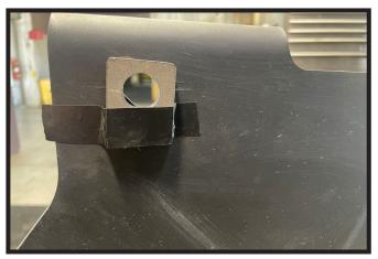
5. Tape the two (2) 1-1/4" x 1-1/2" spacer plates to the outside of the receiver hitch lining them up with the existing hole. Do this on both sides of the hitch.
